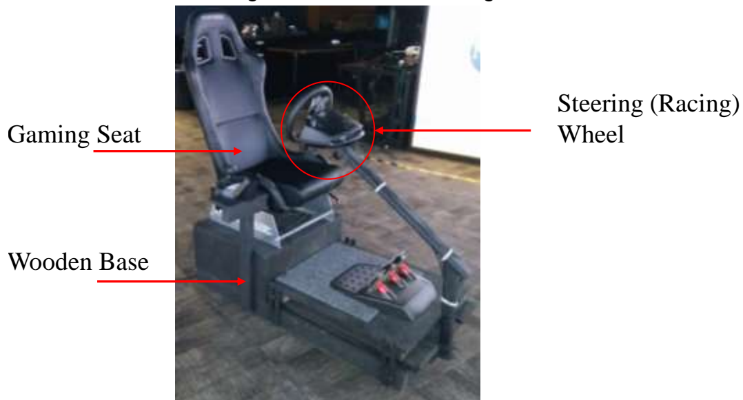
Figure 1: Modified Gaming Seat and Gaming Steering Wheel Utilized to Develop VR-Based Driving Simulator.
