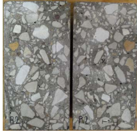
Figure C.1b: Rodded cylinder 2 sawed
