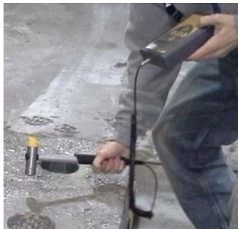
Figure 9: Photograph of the Nitto hammer in use.
