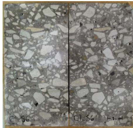
Figure C.1b: Core 1 (Slab 6) sawed
