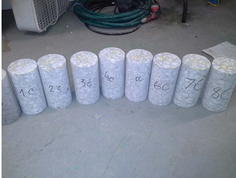
Figure 6: Picture of eight cores extracted from one of the slabs.
