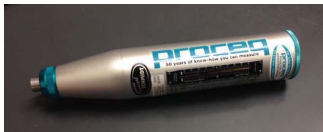
Figure 8: Photograph of the rebound hammer.
