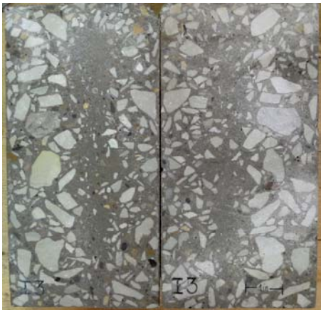
Figure C.1c: Internally vibrated cylinder 3 sawed
