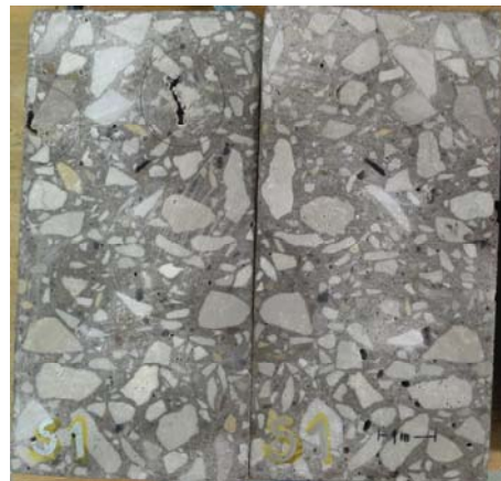
Figure C.1e: Sleeve vibrated cylinder 1 sawed
