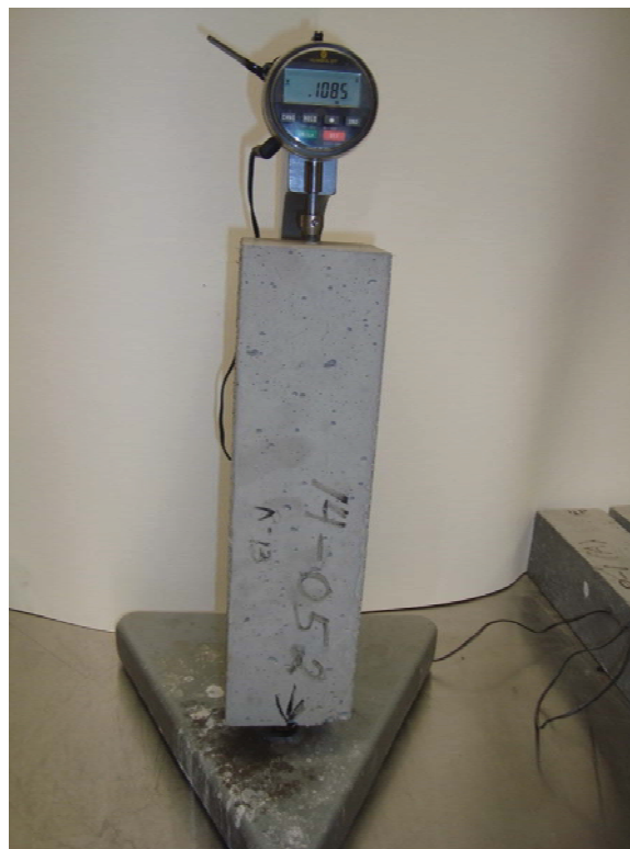
Figure 3.1. Photo - Length comparator used to measure shrinkage of 4" x 4" x 11 1 / 4 " concrete bars in accordance with ASTM C157/C157M - 08(2014) Standard Test Method for Length Change of Hardened Hydraulic-Cement Mortar and Concrete.
