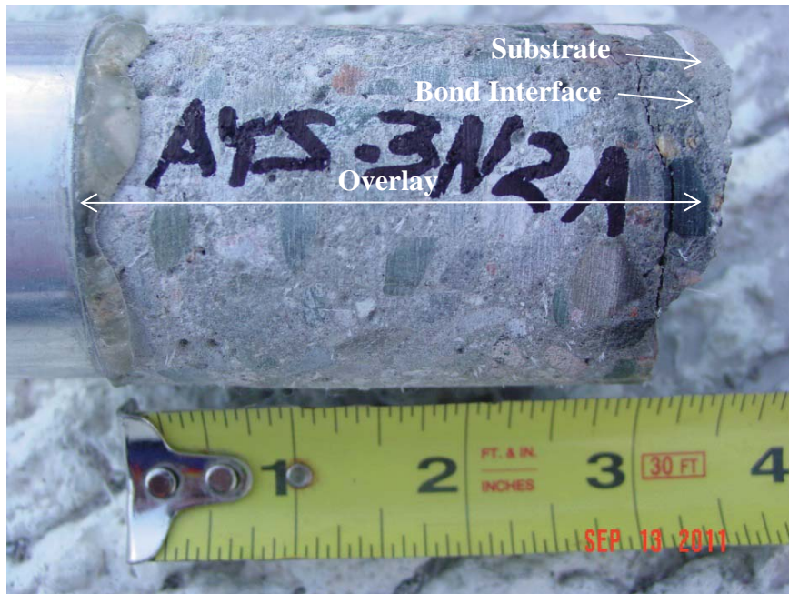
Figure 2.5. Photo - Side view of pull-off test for AYS-3N2A as shown in Table 2.5 in Section 2. Measured pull-off strength was 181 psi.
