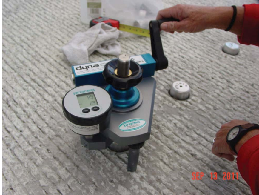
Figure 2.3. Photo - Rotating the crank applied the tensile or pull-off load to the aluminum disk. The digital gauge recorded the maximum load applied.
