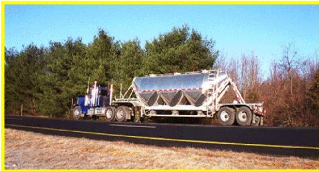
Figure 7A: Air Ride Suspension, Bulk Hauler (Class 9) Vehicle Used During Calibration, October 1998
