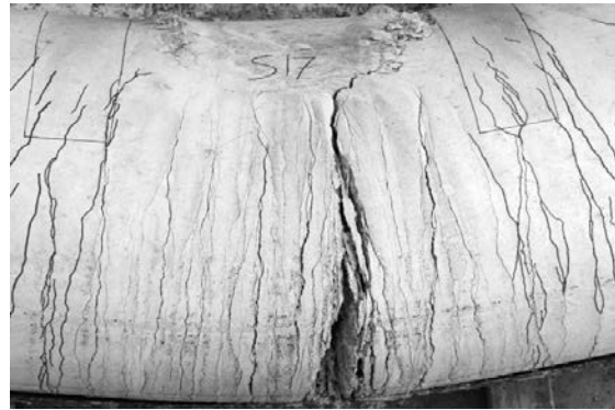
b) Flexural Cracking of Concrete Fill
