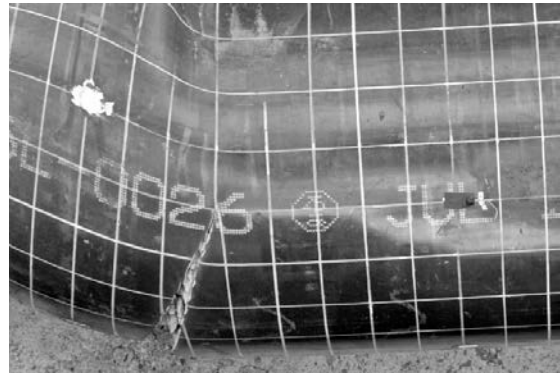
b) Tearing of Steel in Shear Zone
