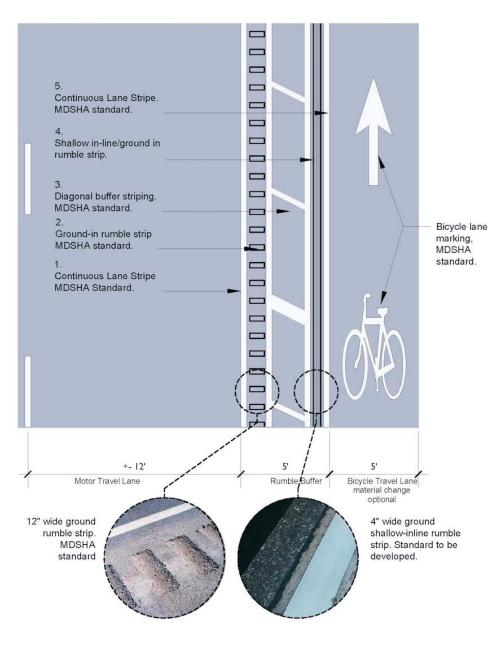
Figure 3 Rumble-buffered bike lane design
