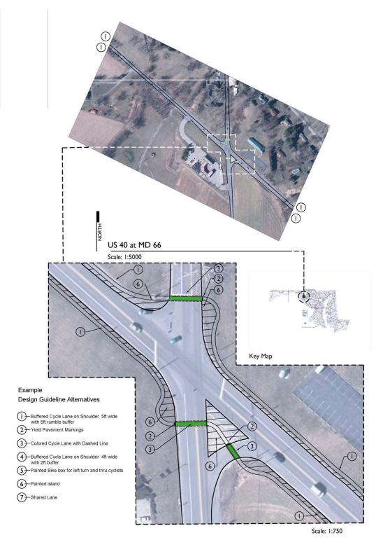
Figure 6b Implementation Study of the At-Grade Intersection of US 40 at MD 66
