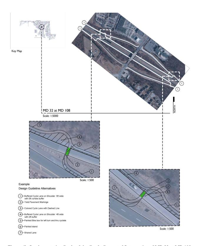
Figure 4b Implementation Study of the Grade-Separated Intersection of MD 32 at MD 108
