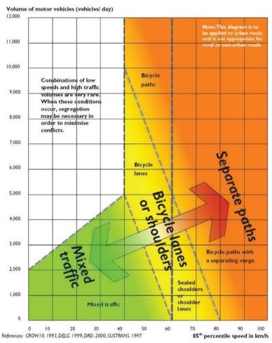
Figure 2-1 Preferred separation of bicycles and motor vehicles according to speed and volume (Source: Austroads AGTM04 2009f)
