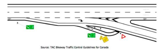
Figure 4-3 Canadian design 1 for diverging ramps
