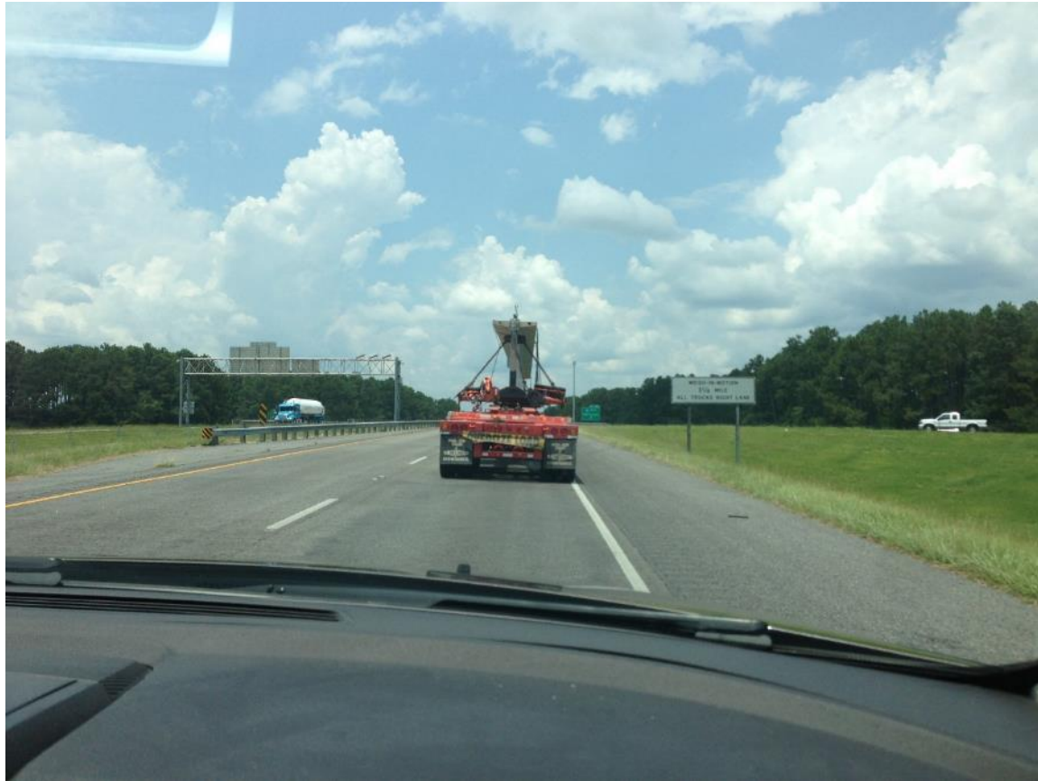
Figure E. 13 View of Girder 1 during Event G1-A3
