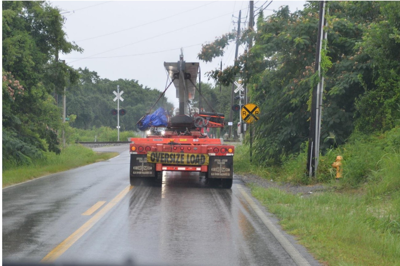
Figure E. 32 View of Girder 1 during railroad crossing
