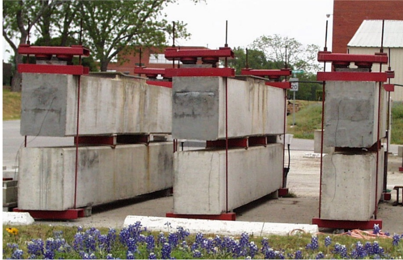
Figure 2.1 Linear Rectangular Beam Specimens (on Top of Reaction Beams) 7
