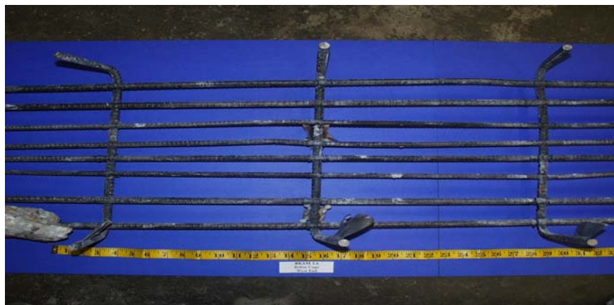
Figure 5.6 Mild Steel Reinforcement Cage
