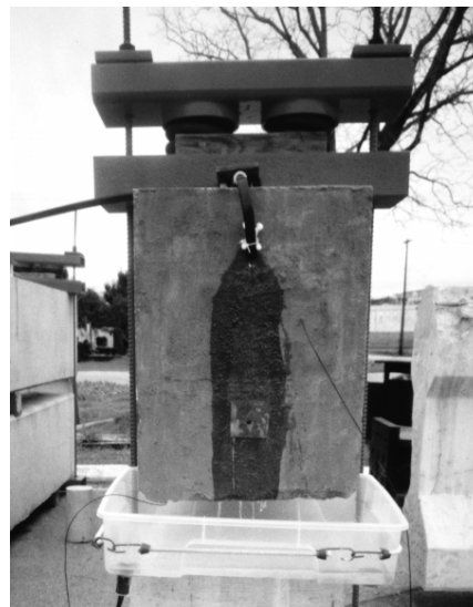
Figure 2.18 Beam End Dripper System 3
