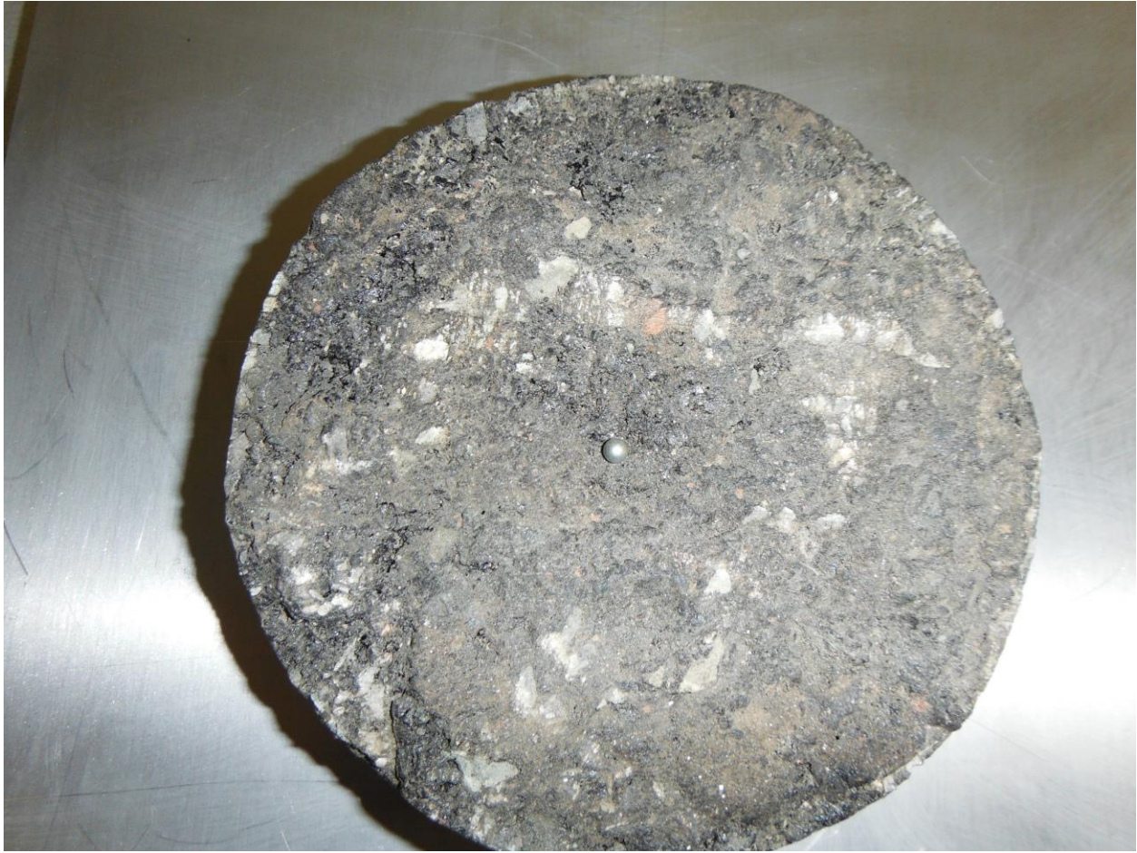
Figure 6. Ball Bearing Placed in Deepest Crevice of Core
