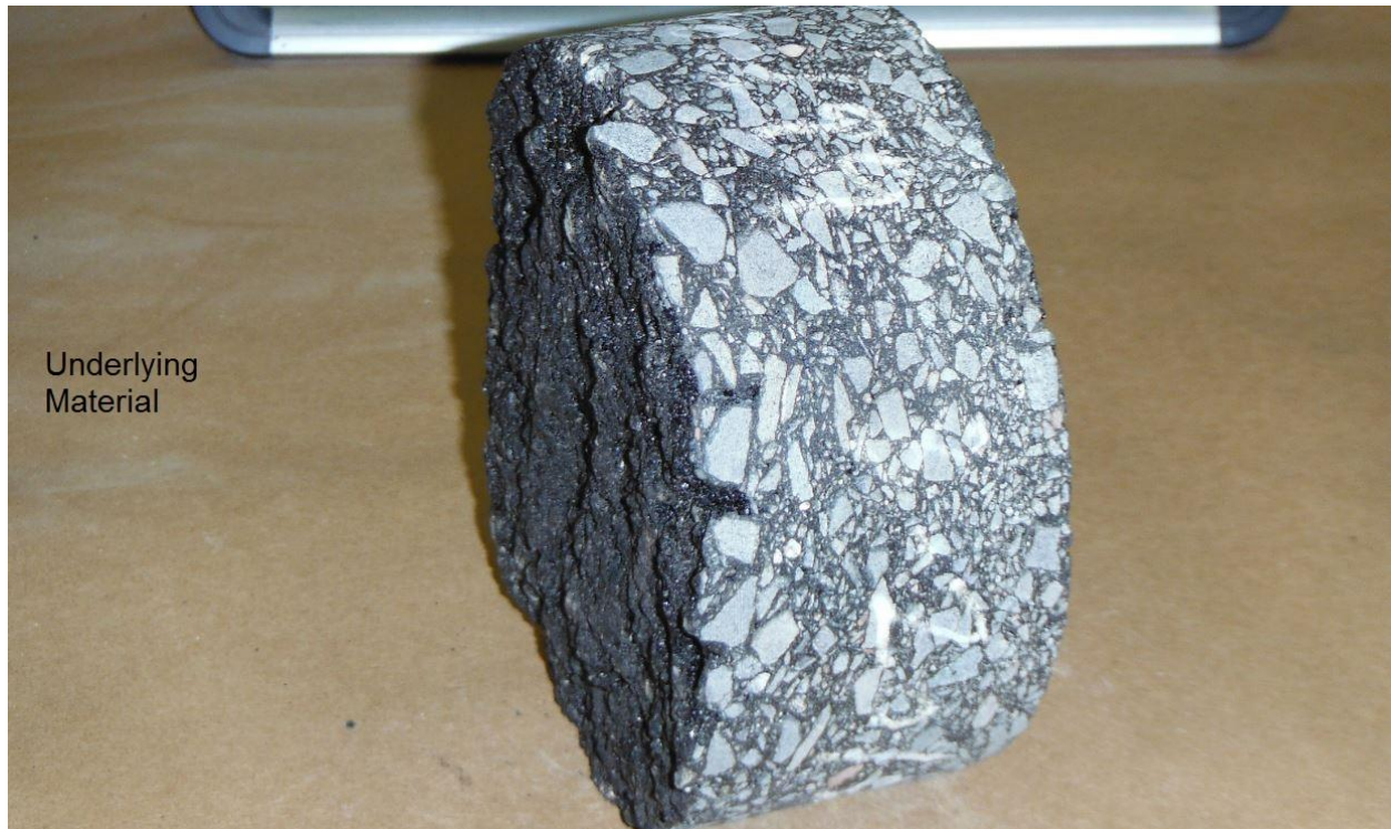
Figure 1. Core with Partial Underlying Layer Attached
