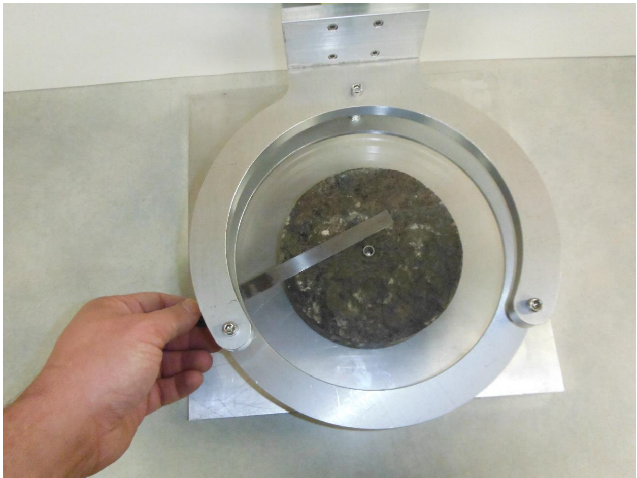
Figure 9. Thin Gauge Metal Used to Determine Glass Plate Contact Point
