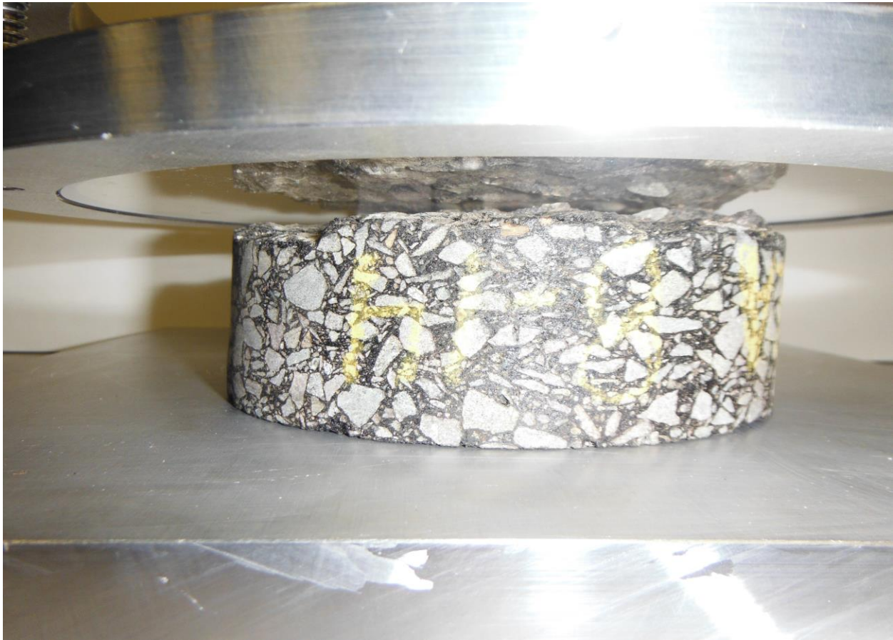
Figure 8. Texture Gauge Glass Plate in Contact With Core
