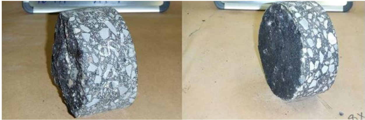
Figure 2. Different Levels of Unclean Separation on Cores
