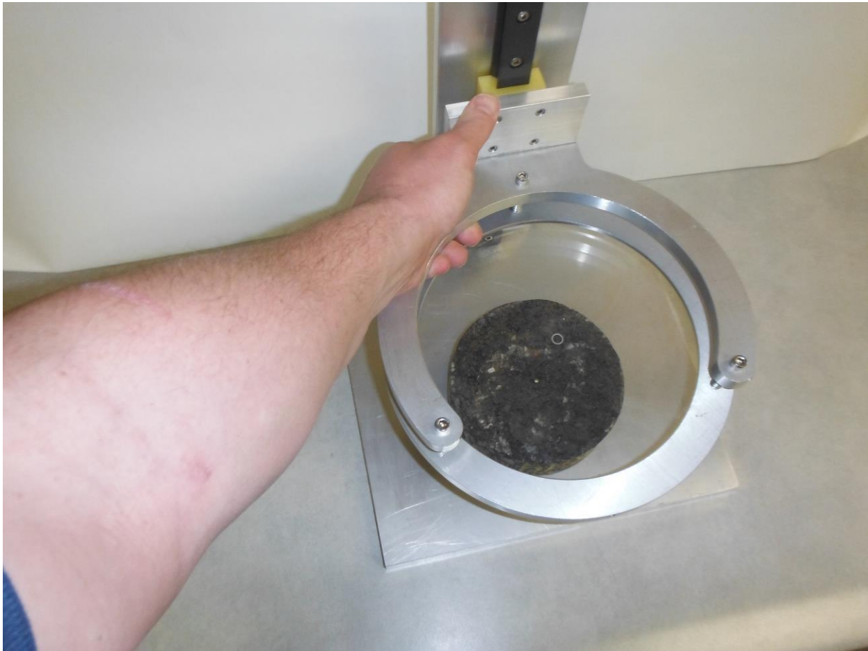
Figure 7. Texture Gauge Glass Plate Lowered onto Core via Slide
