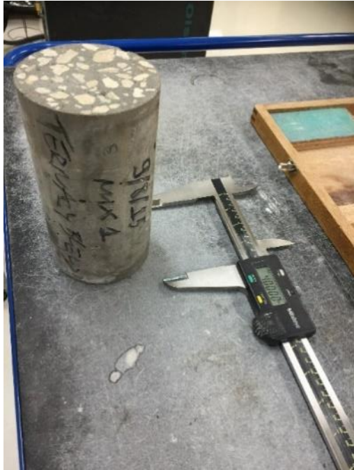
Figure F-8. Specimen measurement and alignment.
