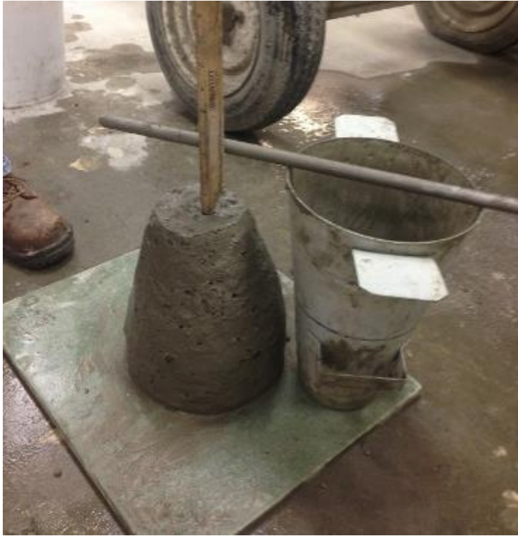
Figure F-1. Performing the slump test.
