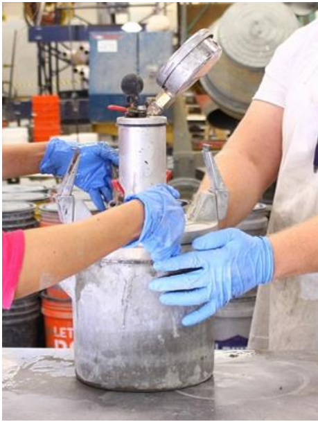
Figure F-4. Air content test. A) air content test apparatus and B) reading of air content.
