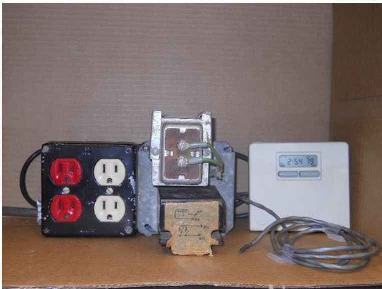
Figure D-5. Switched outlet, transformer, thermostat, and relay used
