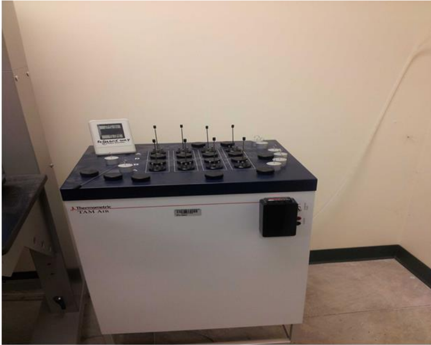
Figure 2-1. TAM Air calorimeter.
