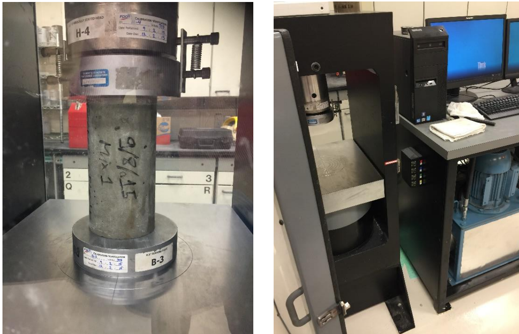
Figure F-6. The Forney testing machine used for the compressive strength testing.
