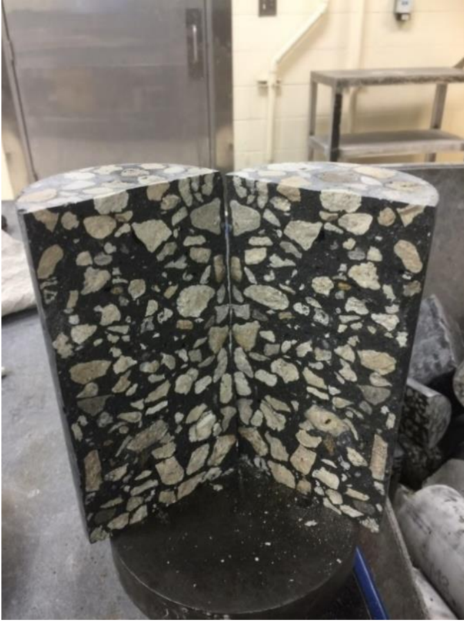
Figure F-12. Splitting tensile strength test specimen after conducting the test.
