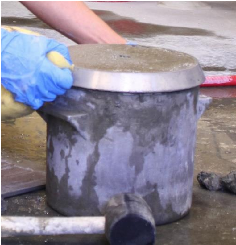
Figure F-3. Conducting unit weight test.
