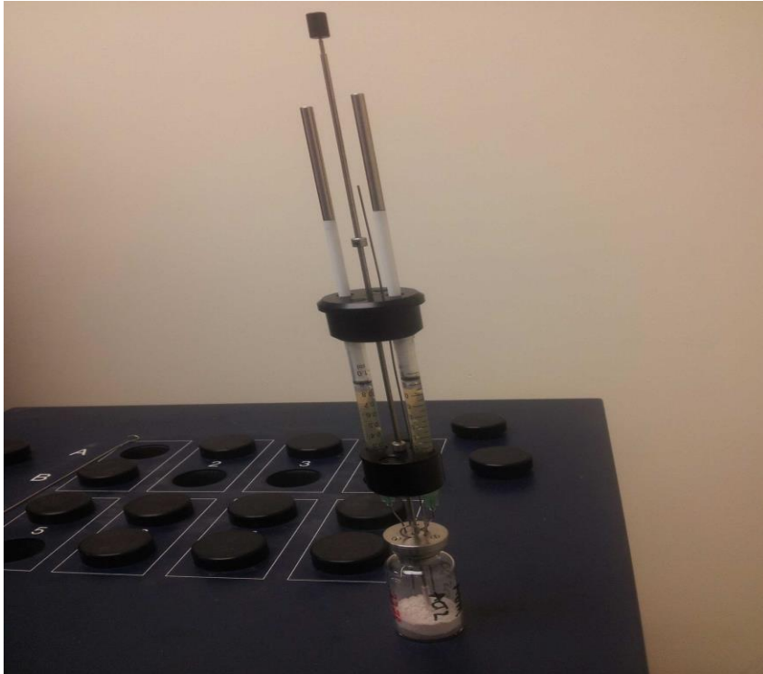
Figure 2-2. Admix. ampoule with the test sample and stirrer-syringe assembly.
