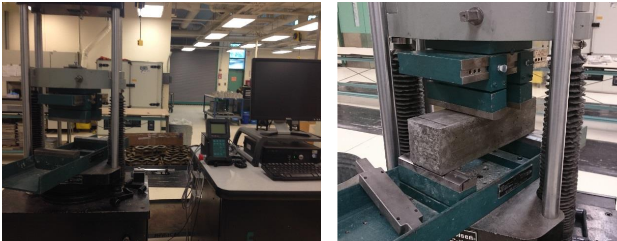
Figure F-13. Testing machine for flexural strength test before and after installing concrete beam.
