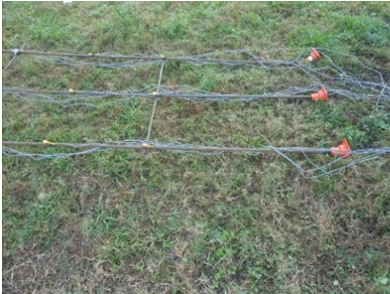
Figure E-3. Temperature loggers attached to steel frame.
