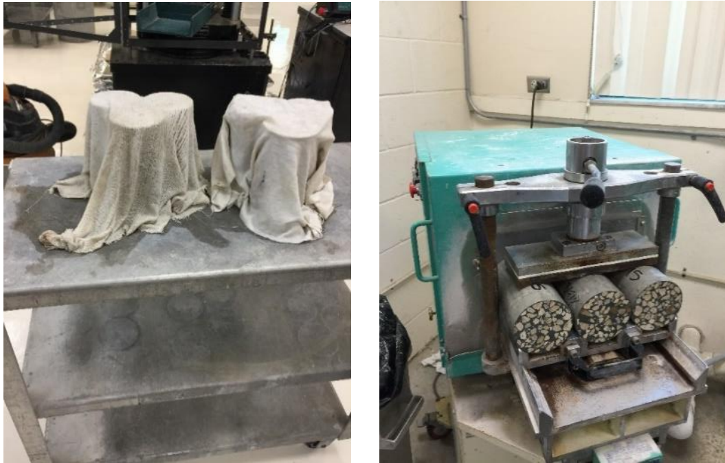
Figure F-7. Grinding each side of the specimens and keeping the specimens moisturized until the test is completed.
