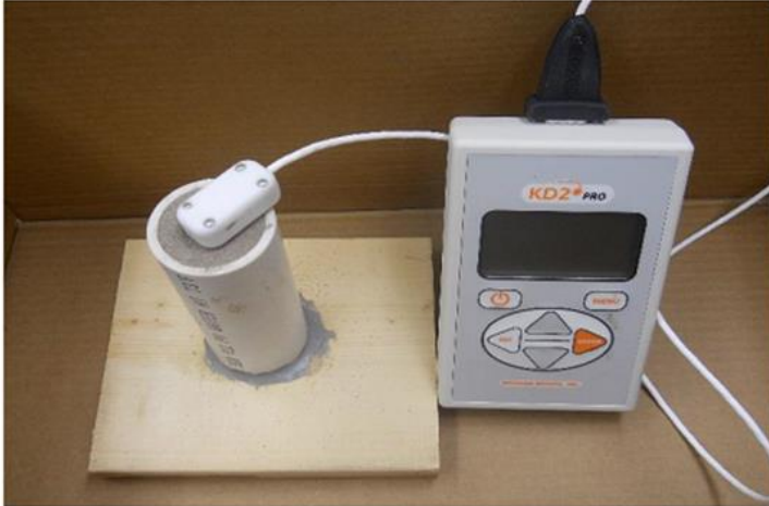
Figure D-9. The PVC pipe with soil sample and TR1 probe in a 75° F testing condition.
