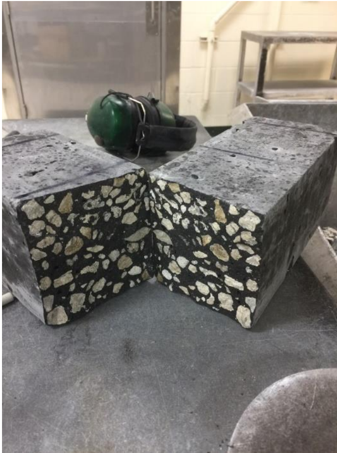
Figure F-14. A fractured flexure beam specimen.
