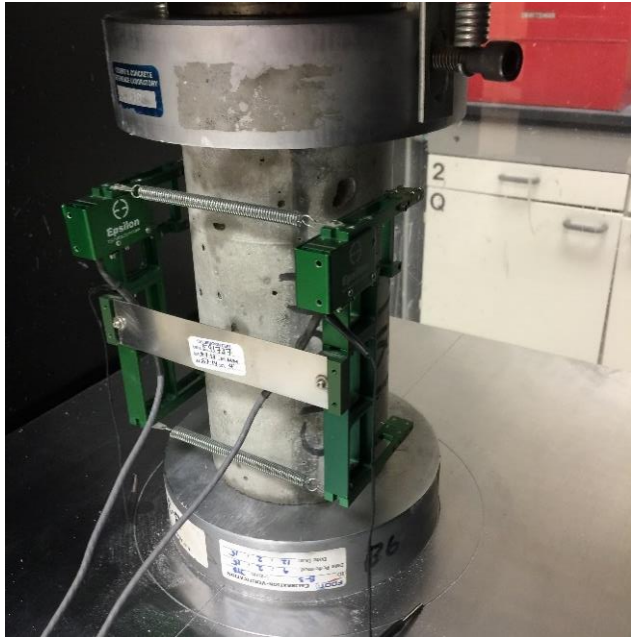
Figure F-10. The compressometer (electronic sensor connected to the Forney software).
