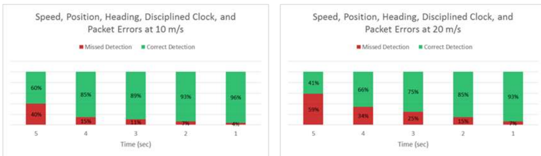
Figure 150: Probability of Misclassification in the Presence of Speed, Positional, Heading, Clock, and Packet Errors (Source: USDOT)
