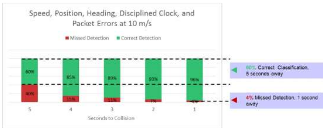
Figure 61: Percentages of with each Resulting Classification from analyzing a pair of Projected Vehicle Trajectories in the Near Miss Scenario; each Second before Collision (Source: USDOT)
