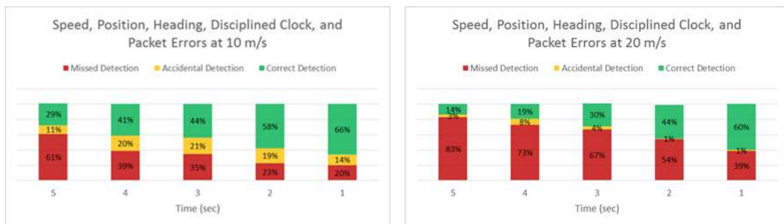
Figure 144: Probability of Misclassification in the Presence of Speed, Position, Heading, Clock, and Packet Errors (Source: USDOT)
