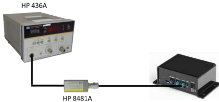
Figure 3: Measuring the Output Power of a DSRC Radio (Source: USDOT)
