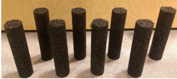
Figure 3-7. FAM specimens: 12 grams (mass), 50 mm long, and 12 mm in diameter.
