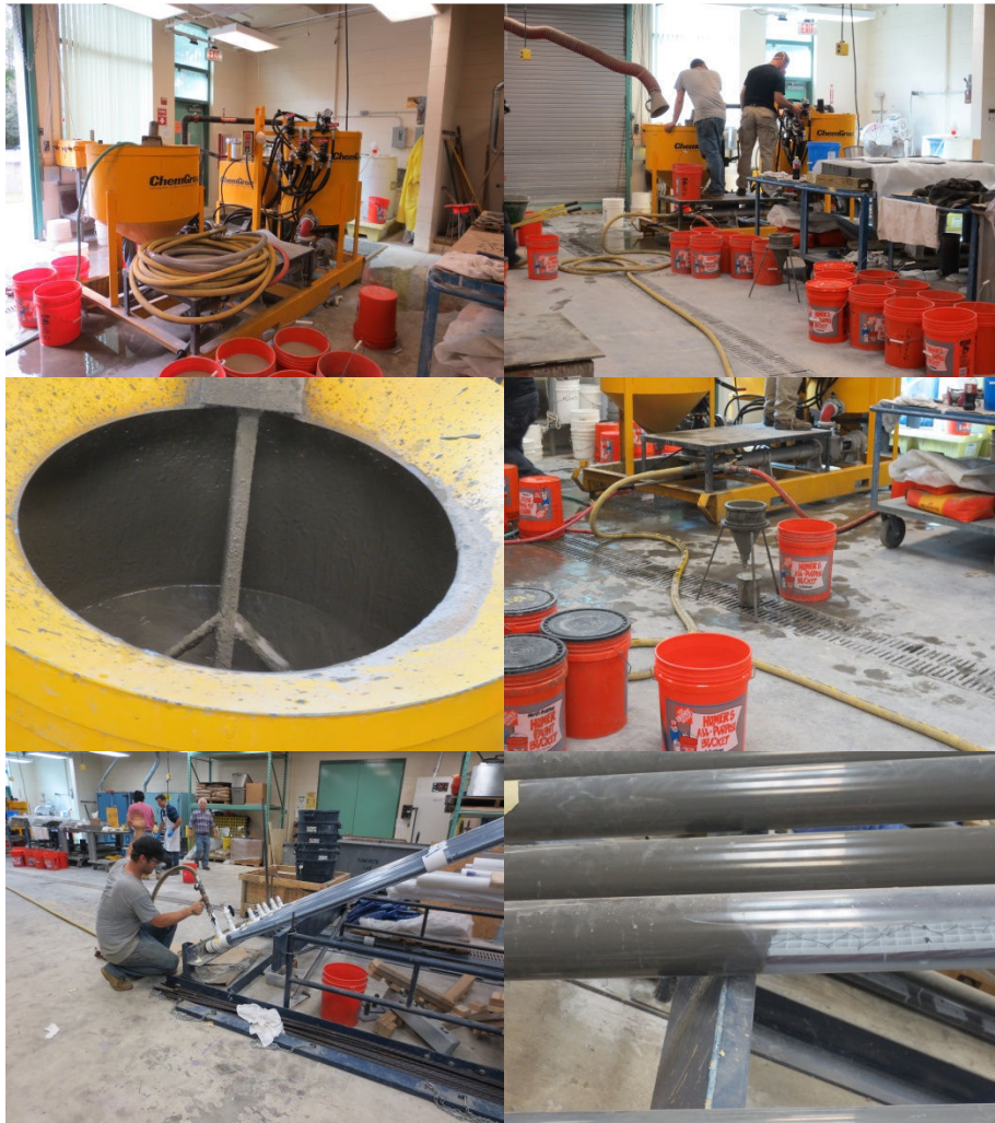
Figure 6.6. Grout batching, mixing, and pumping sequence.
