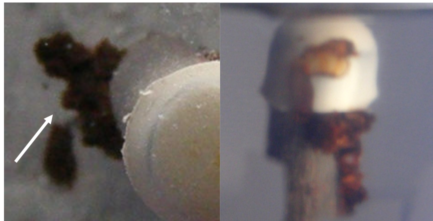
Figure 2.21. Solid corrosion product on steel in 0.13% sulfate solution, pH 12.6. Photos of samples submerged in solution. (From Lau et al., 2013b.)
