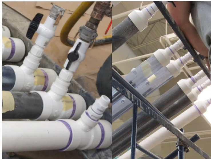
Figure 6.1. Assembled PVC inlet and outlet fittings. Left: Inlet. Right: Outlet.
