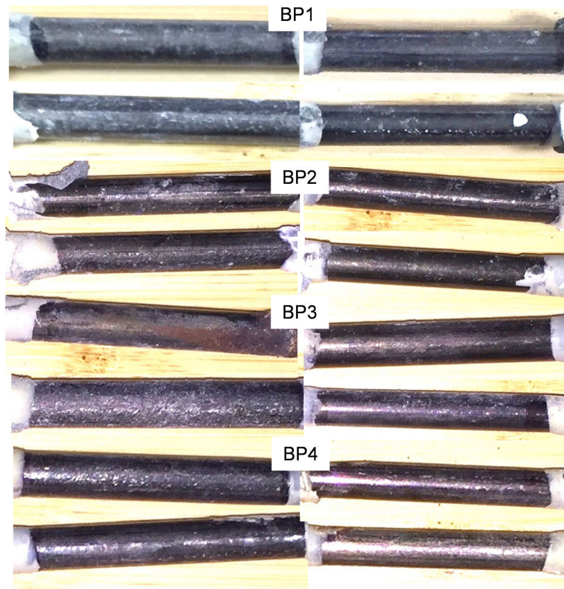
Figure 8.5. Photos of steel wire from INT samples (Cases BA1-3).
