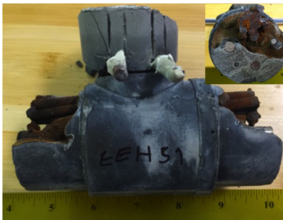
Figure 5.3. Case B.P.4.1 after ~300 days from casting. (Corrosion product appear after exposure to the ambient lab air)
