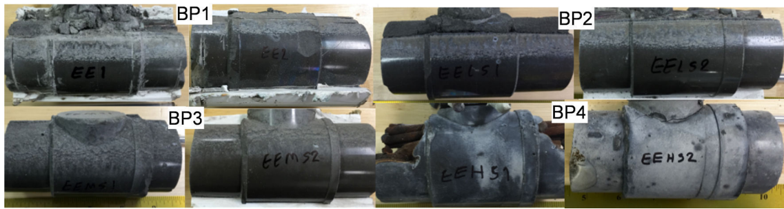
Figure 7.8. Photos of grout in tee body from INT test samples cast with pre-exposed Grout B. (Cases BP1-4)
