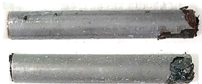
Figure 4.7. Corrosion development of steel in pH 12.6 sulfate solution (20,000 ppm Na 2 SO 4 , 30-Min Cathodic Pre-Conditioning).
