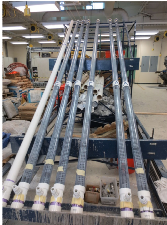
Figure 6.3. Assembled MIT test samples supported at incline for grout injection.
