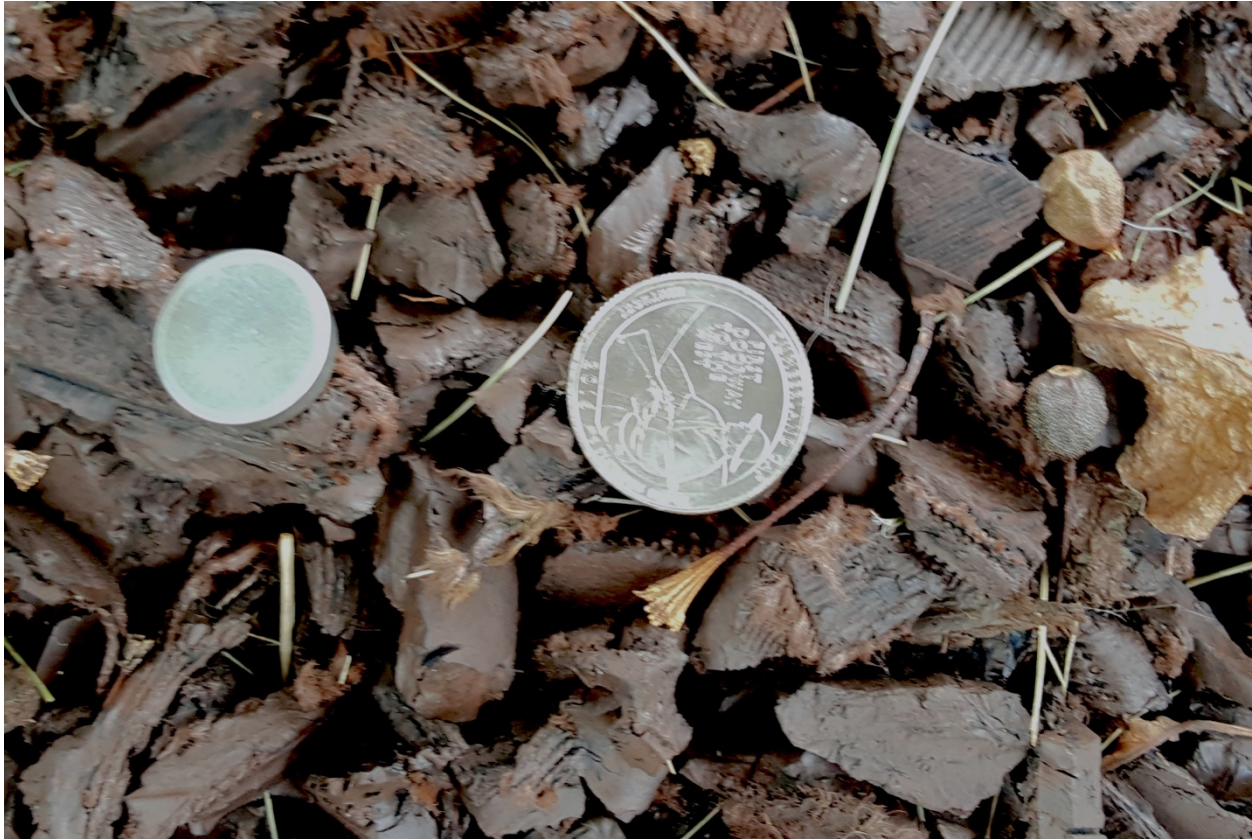
Figure 2.12. Photograph of “iButton” (left) used to monitor nest temperatures of Northern Map Turtles. A quarter is shown on the right to indicate scale.
