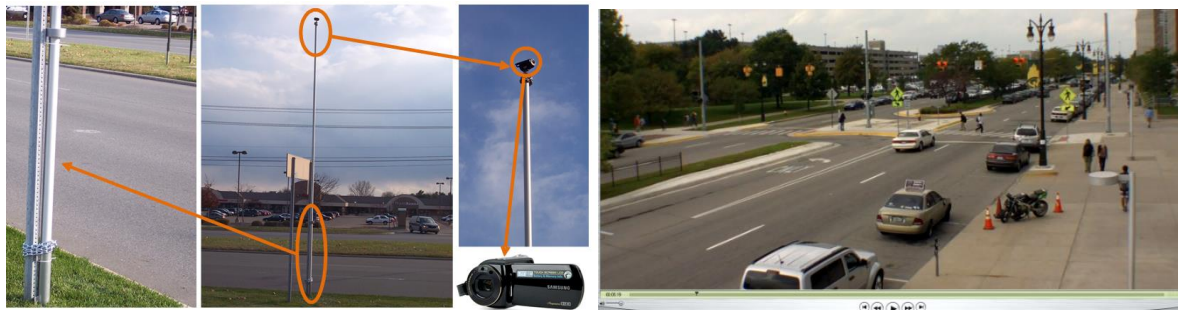
Figure 1. Typical Video Camera Setup for Recording Motorist Yielding Behavior
