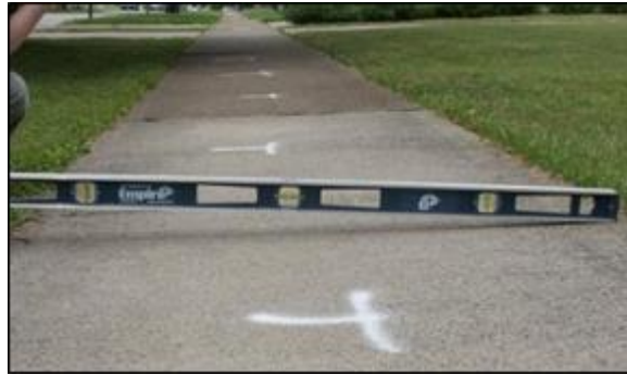
Measuring Cross Slope 3
