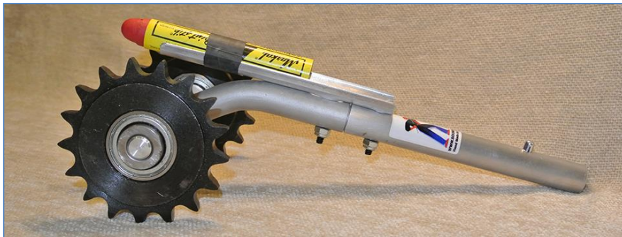
Figure 5: Delam 2000 rotary percussion tool for detecting shallow delaminations
