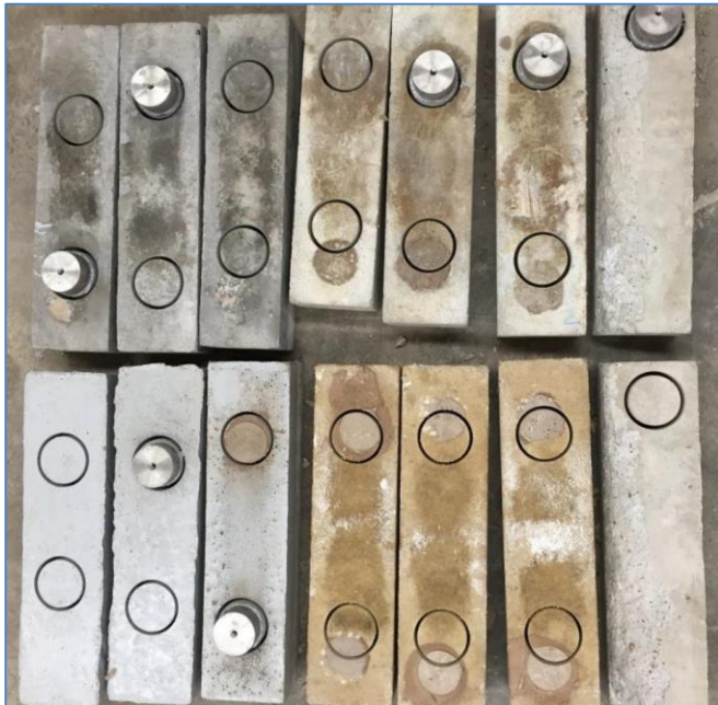
Figure 11: Bond testing of two layer specimens following freeze thaw testing (Amini 2015)
