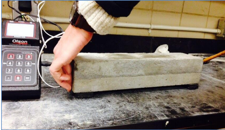
Figure 9: Two layer bonded specimen and ASTM C215 resonance testing (Amini 2015)
