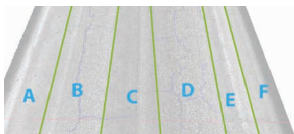
Figure 2.1 Longitudinal sections in a pathway. (Courtesy of Pathway Services Inc.)
