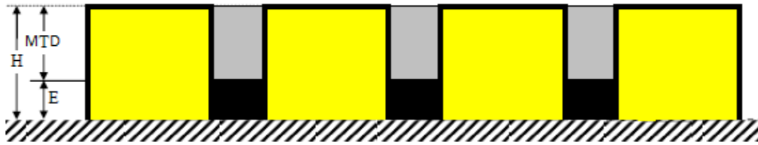
Figure 5.1: Embedment depth calculation according to NCHRP 680
