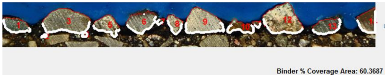
Figure 4.15: Aggregate surface coverage
