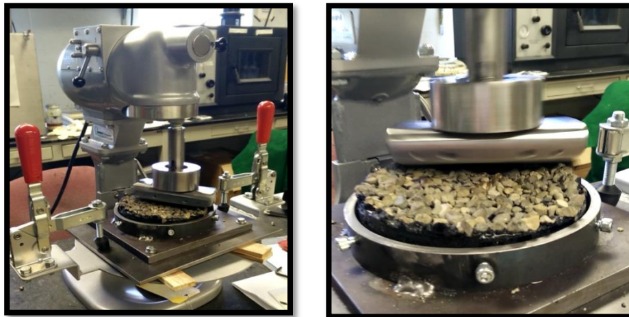
Figure 5.4: Sweep test procedure on chip seal surface
