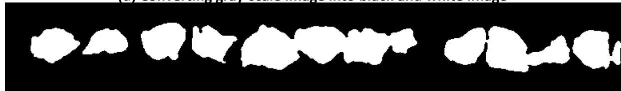
(e) Filling the holes on the aggregate surface
