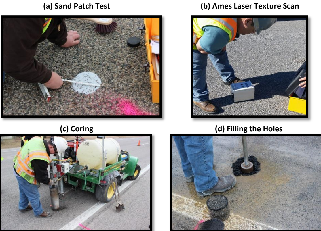
Figure 3.3: Procedure for taking cores from the field
