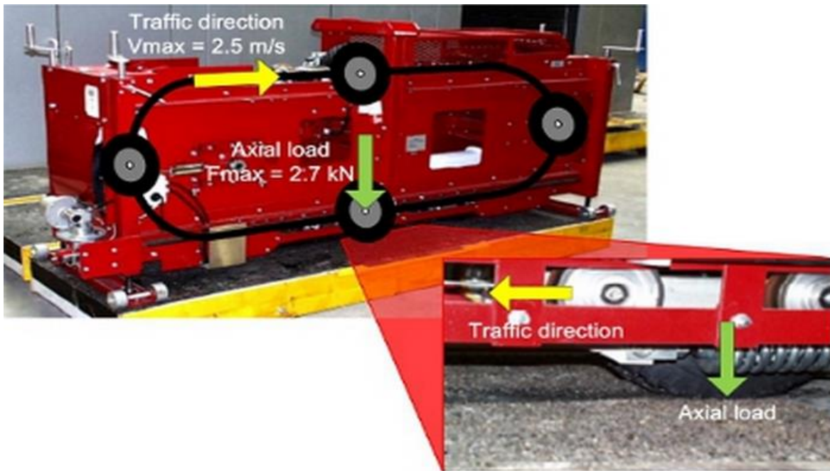
Figure 2.9: The Third Scale Model Mobile Load Simulator (MMLS3)
