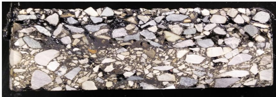
Figure 6.1: Double chip seal cross section
