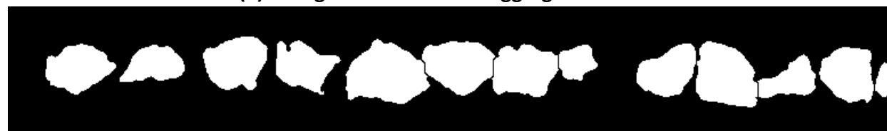
(f) Watershed transform application to separate aggregates
