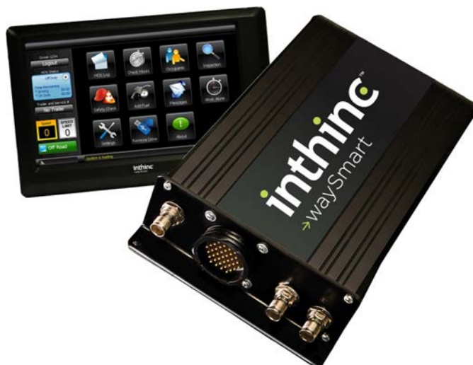
Figure 1. Photograph. The tested OBMS driver interface and controller unit hardware.
