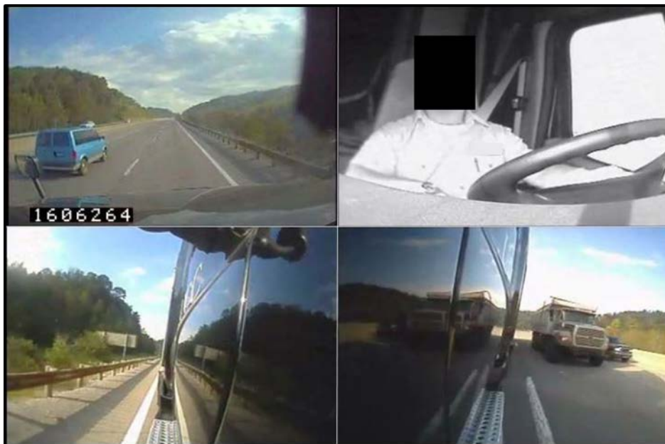
Figure 5. Photograph. Four camera images multiplexed into a single image.
