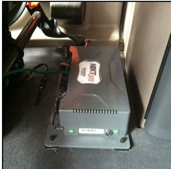
Figure 2. Photograph. The NextGen DAS positioned behind the passenger seat.
