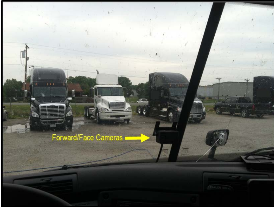
Figure 3. Photograph. DAS forward and face camera mounted on windshield.
