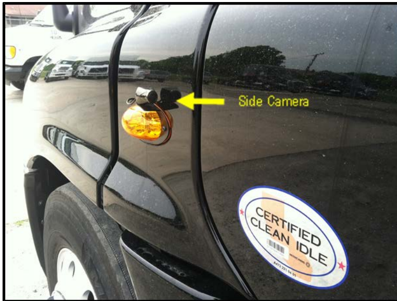
Figure 4. Photograph. DAS driver-side, rear-facing side camera mounted on fender.
