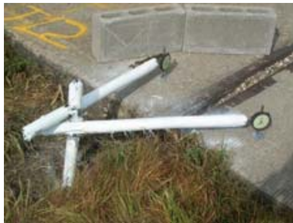
Figure 4.9 Dial indicator used to measure curling at ends of PCP slabs
