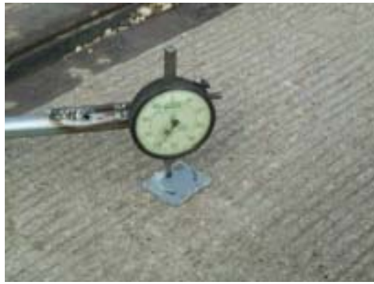
Figure 4.9 Dial indicator used to measure curling at ends of PCP slabs
