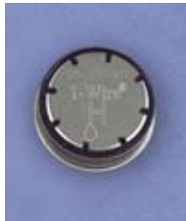
Figure 7.9 Hygro-Button used for measurement for moisture in concrete
