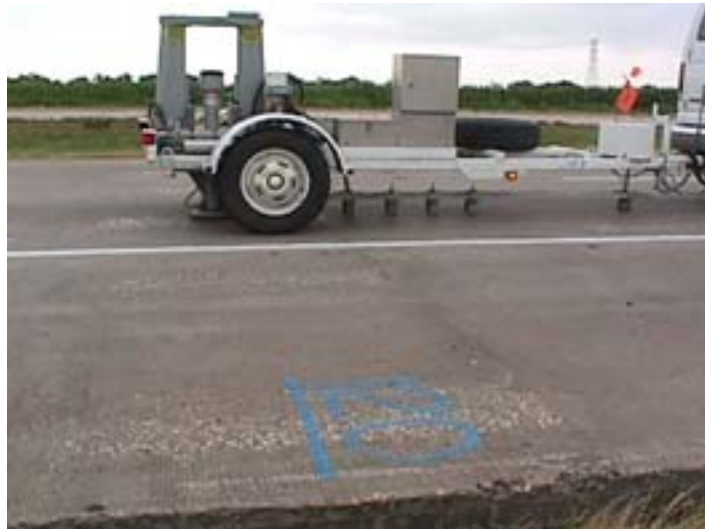
Figure 7.4 FWD loading plate and arrangement of geophones
