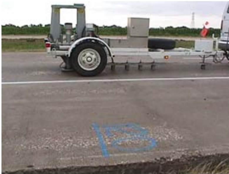
Figure 4.13 FWD equipment used for deflection measurement
