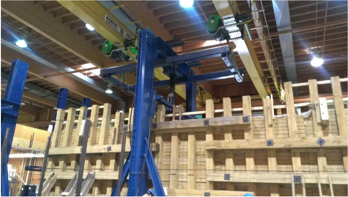
Figure 3. Side Elevation View of Soil Confinement Box and Load Frame
