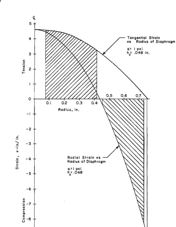
Fig 9. Graphical representation of strains measured by diaphragm strain gage.
