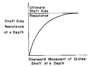
Fig 2a. Shaft side resistance developed at a depth as a function of shaft movement.
