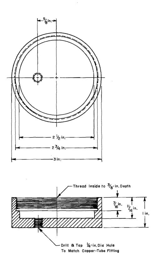
Fig 17. Hydraulic calibration chamber.
