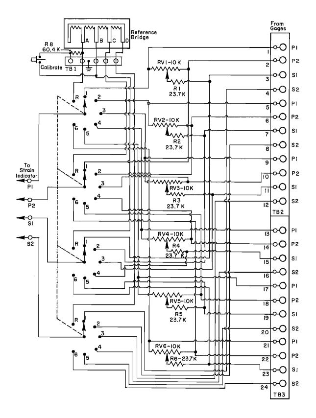
Fig C.1. Six-channel switch and balance unit.
