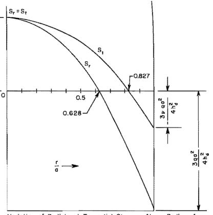
Variation of Radial and Tangential Stresses Along Radius of Uniformly Loaded Circular Diaphragm with Clamped Edges
