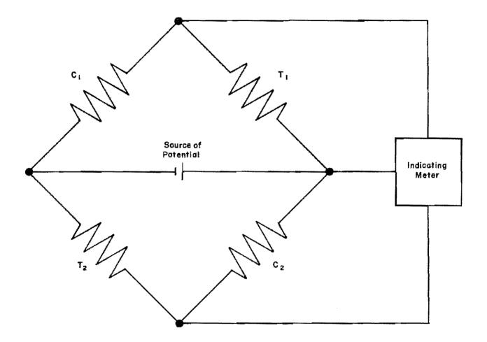
compensation may be obtained automatically by maintaining opposite arms of the bridge at the same temperature. The full-bridge circuit provides certain advantages over the half-bridge circuit, even though both will provide temperature stability. Advantages include double sensitivity and elimination of adverse effects of extraneous resistance changes in cable conductors (Ref 10).
