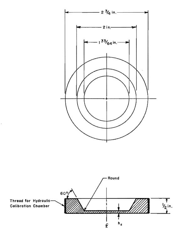
Fig 6. The UT lateral earth-pressure cell.
