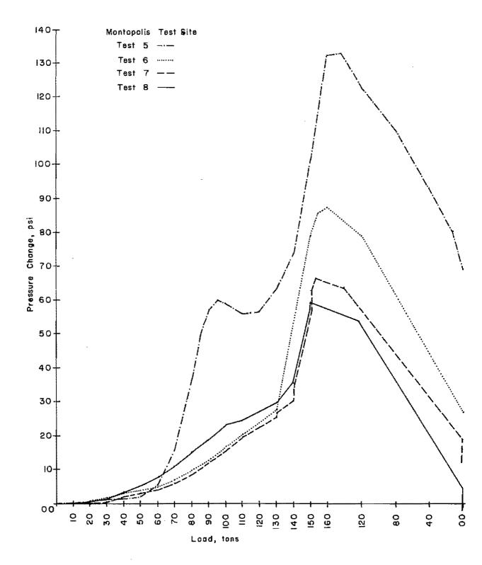
Fig D.2. Behavior of Cell No. 2 during load tests at 10-foot depth in Austin shaft.
