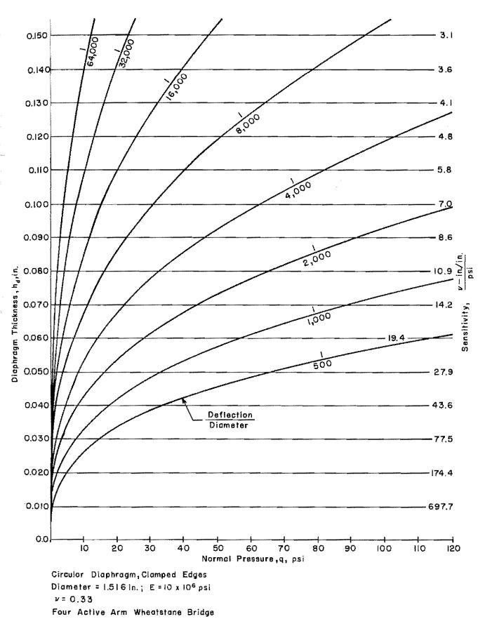
Fig 12. Design map for aluminum cell.
