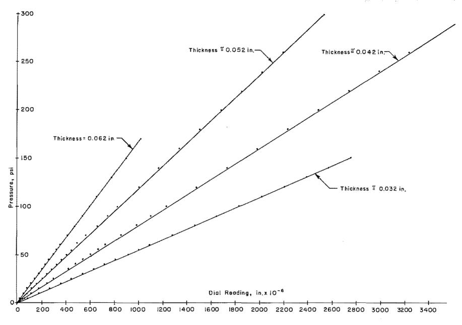
Fig 14. Calibration curves for steel test cell.
