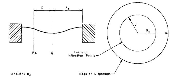
Fig 7. Clamped-edge-diaphragm behavior under uniform load.
