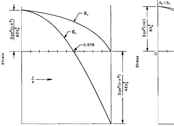
Distribution of Radial and Tangential Strain on Uniformly Loaded Circular Diaphragm with Clamped Edges
