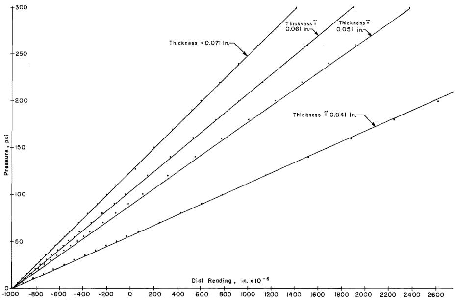
Fig 13. Calibration curves for beryllium-copper test Cell No. 1.
