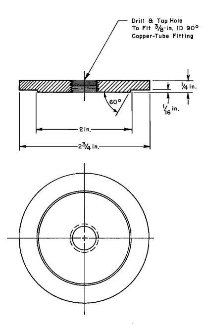
Fig 34. Back coverplate for UT cell.
