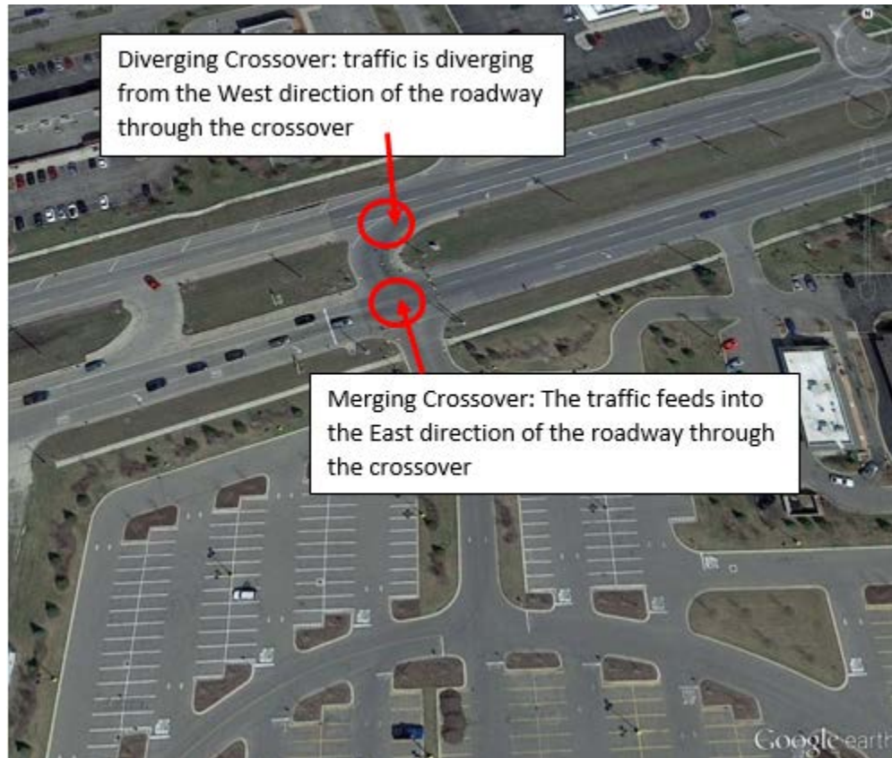
Figure 5. Screenshot of a crossover on a 4D segment
