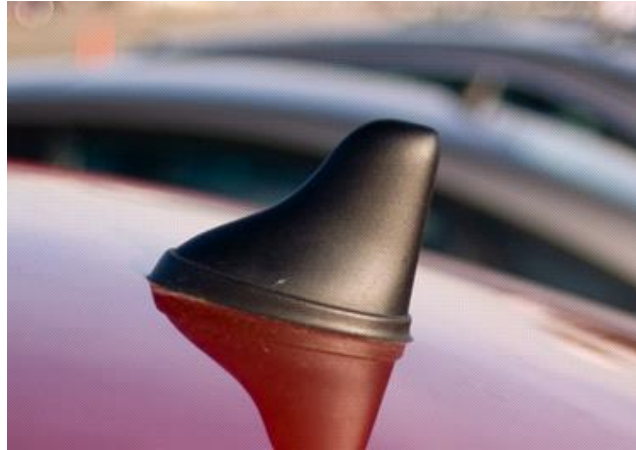
Figure 11. Hirschmann shark fin combined DSRC/GPS antenna.
