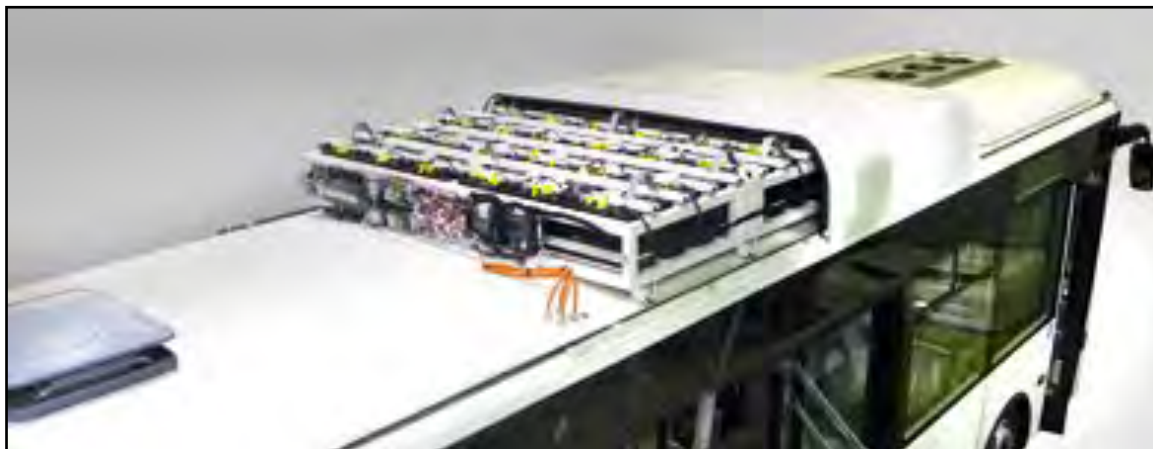
Figure 10. Battery Pack on the Roof of the Bus
