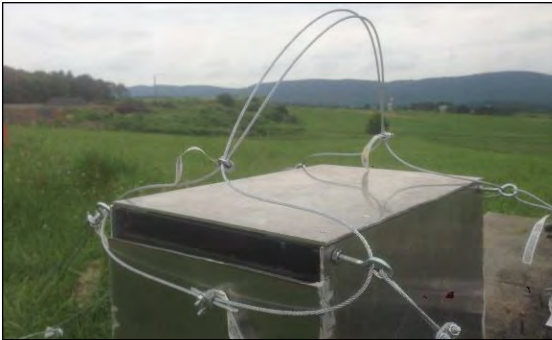
Figure 86. Handle to Lift the Battery Pack up with the Forklift
