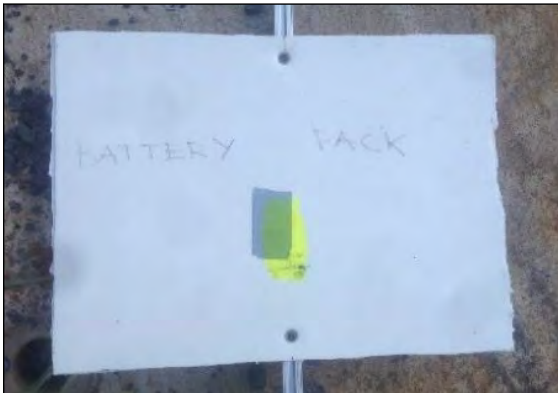
Figure 108. Impact Accuracy of Pendulum to Battery Position
