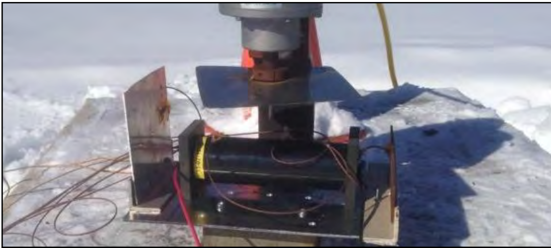
Figure 42. Acetal Overcharge with Blast Shield Material Test Setup
