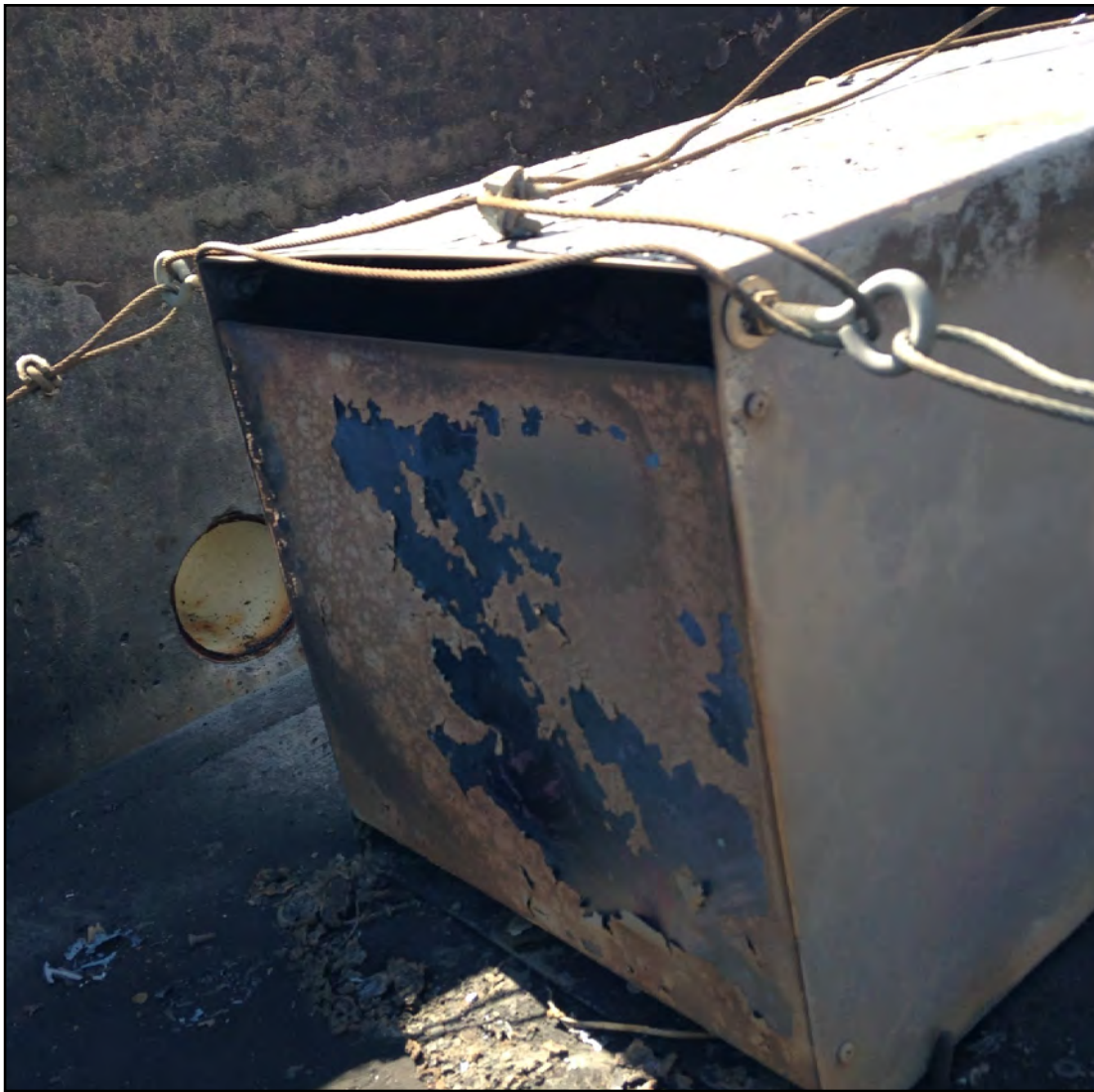
Figure 101. Resulting Steel Module Enclosure
