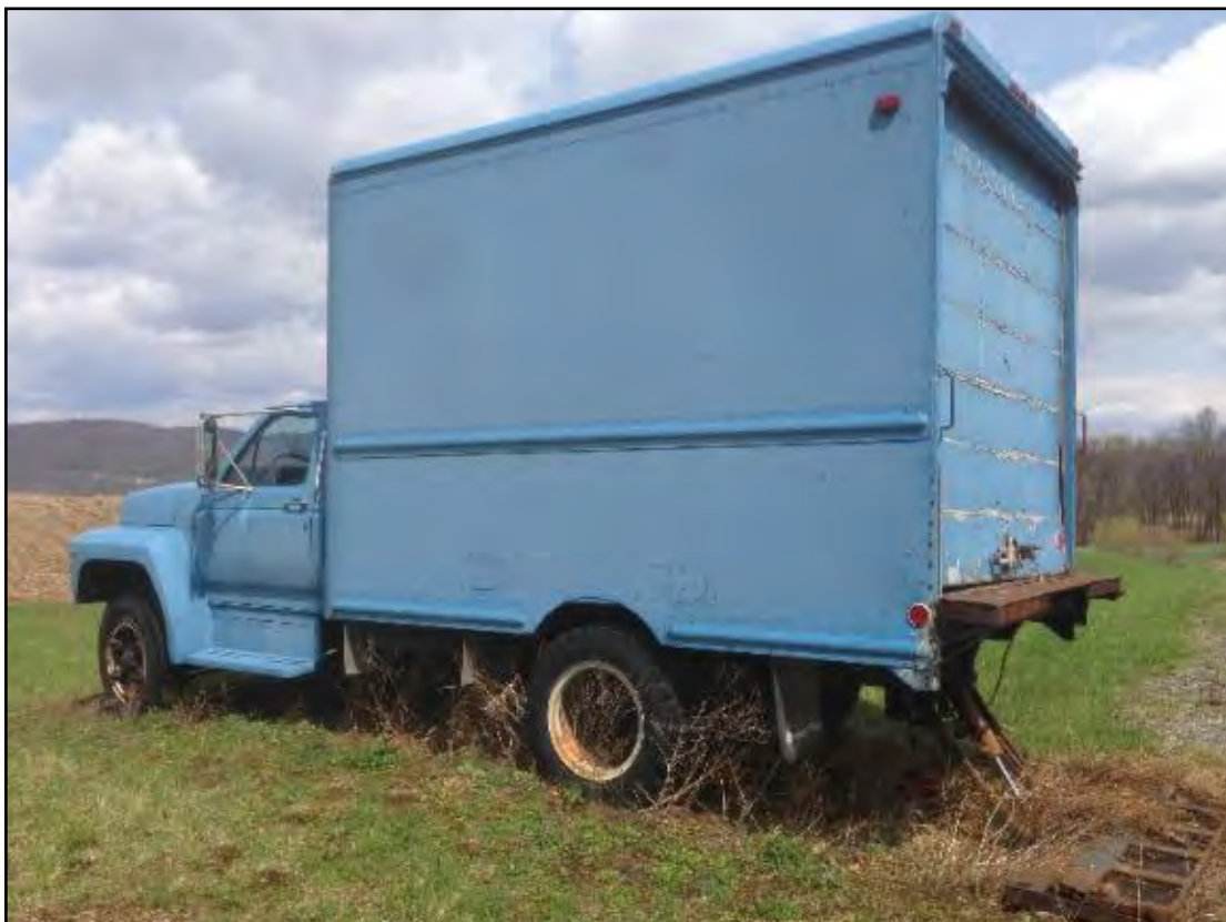
Figure 102. 18,400-lbs. GVWR Refrigerated Truck to Simulate Bus
