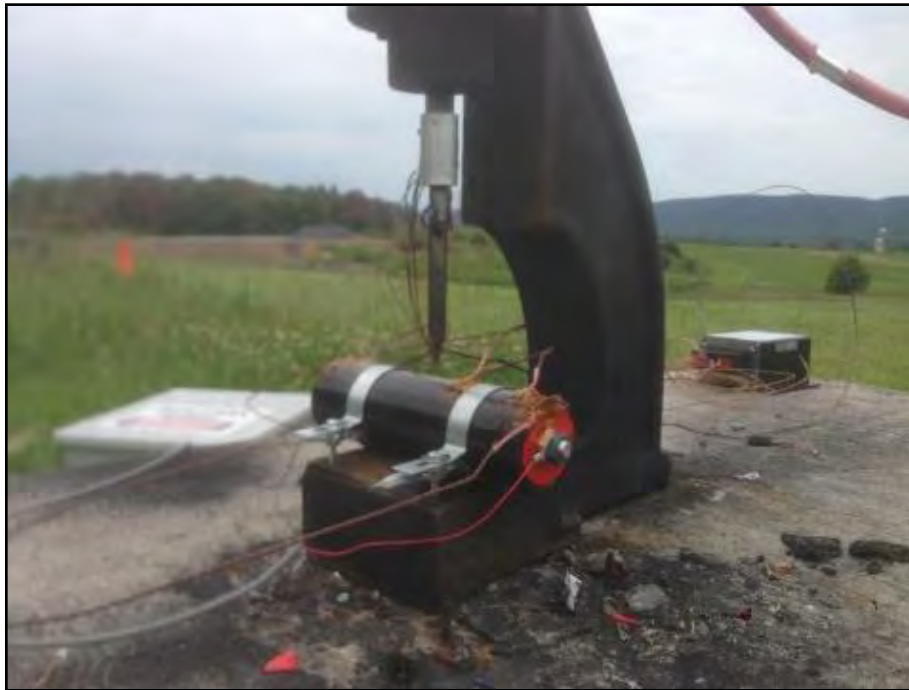
Figure 72. Nail Tip Temperature Measurement Test Setup
