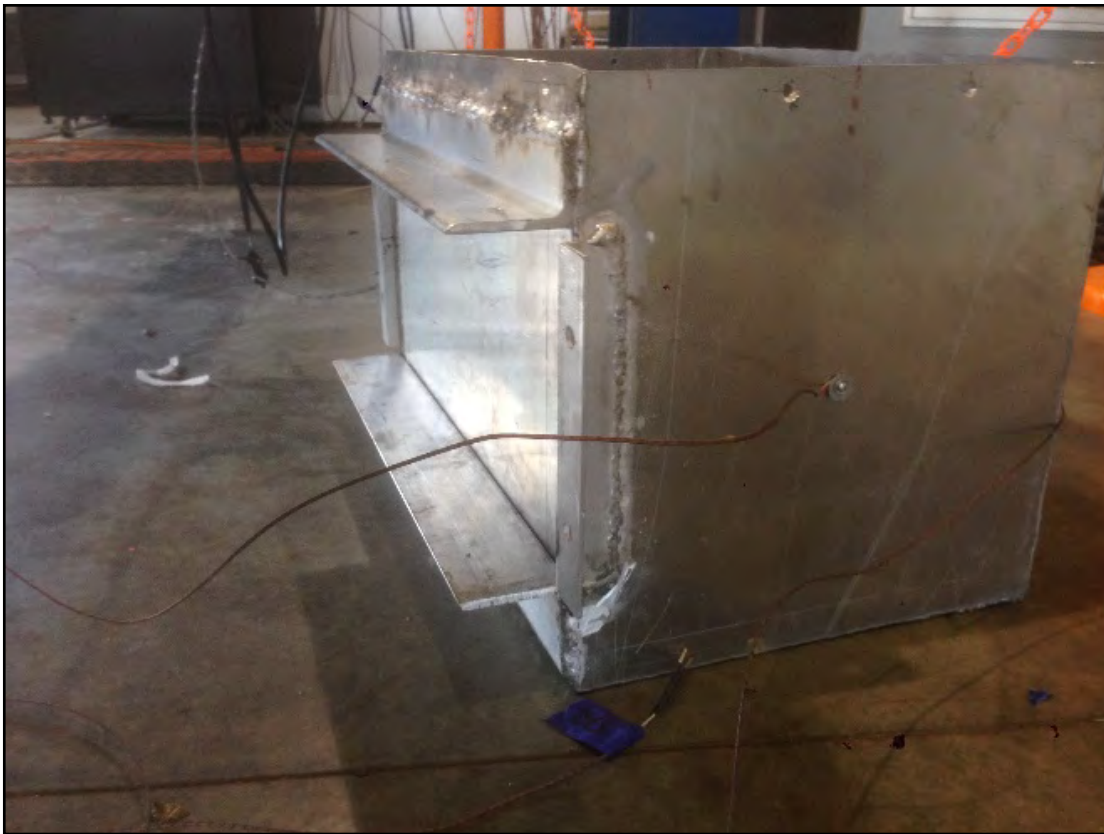
Figure 109. Aluminum Enclosure with Frame Mounting Flanges
