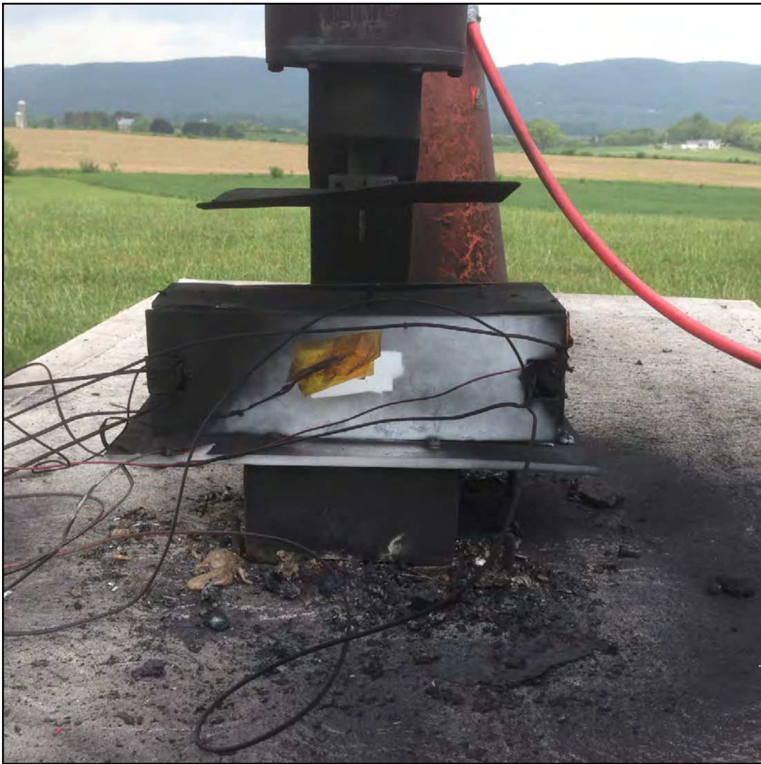
Figure 71. Teflon – Nail Puncture Material Results
