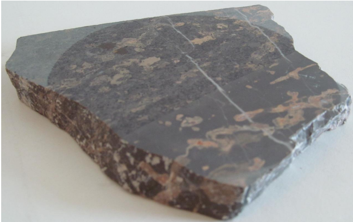
Figure 4.5 Prepared sample from Dolese Cooperton (limestone)
