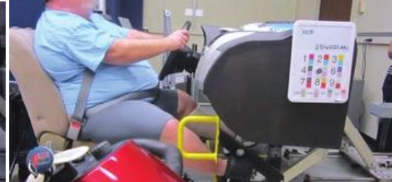
Figure 24. Photos showing lap belt fit for a range of occupant sizes (stratified by BMI classification).
