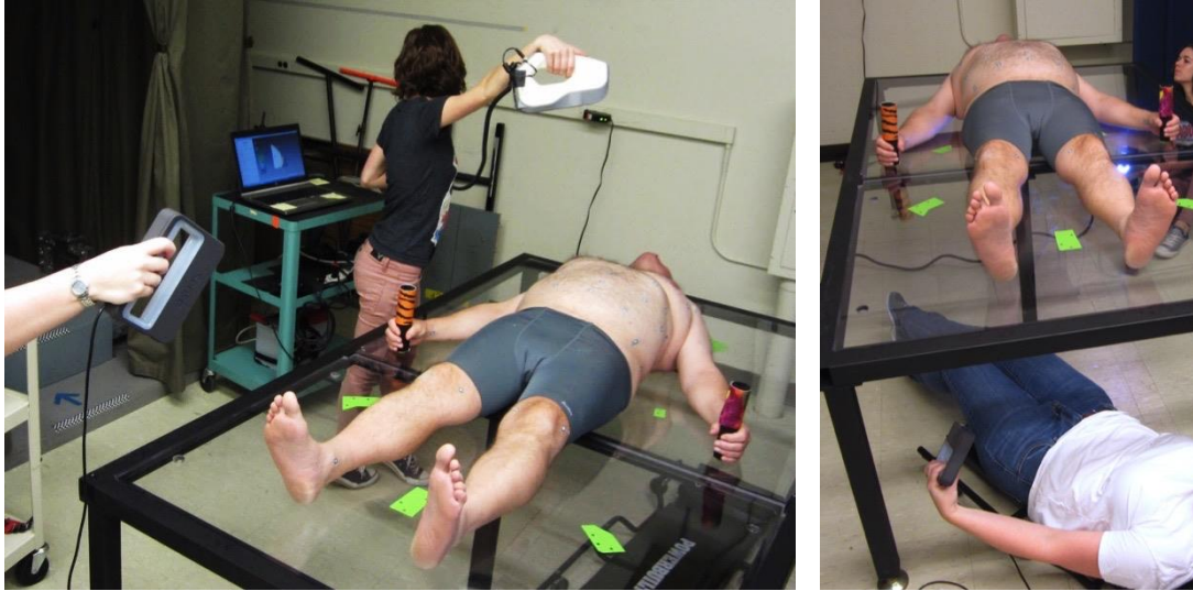
Figure C30. Recording scanning supine posture with Artec and Sense scanners on participant's anterior (left) and posterior (right)
