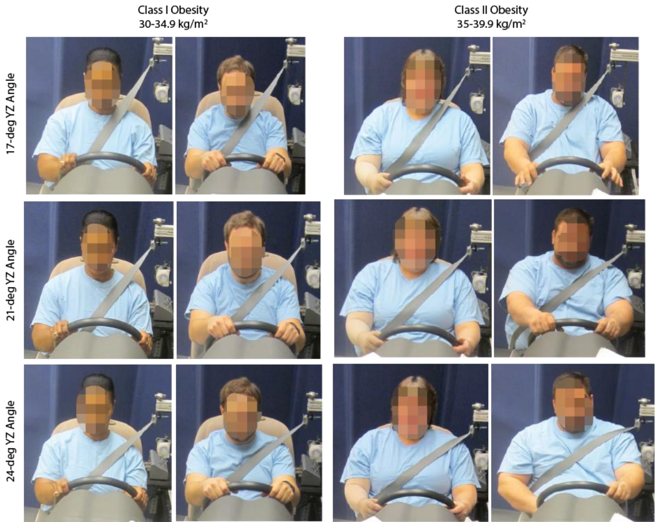
Figure 32. Photos showing shoulder belt fit for a range of occupant sizes.
