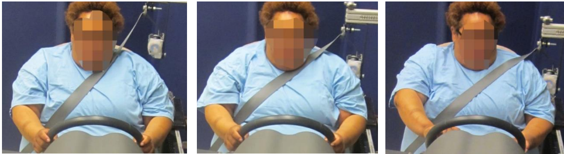
Figure 31. Example of belt fit for participant (BMI=55.3 kg/m 2 ; Stature=1633mm) for anchorage locations YZ angles of 17, 21, and 25 degrees (left to right).
