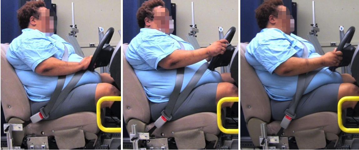
Figure 23. Example of belt fit for a participant (BMI=55.3 kg/m 2 ; Stature=1633mm) for anchorage locations 30, 52, and 75 degrees to horizontal (left to right).
