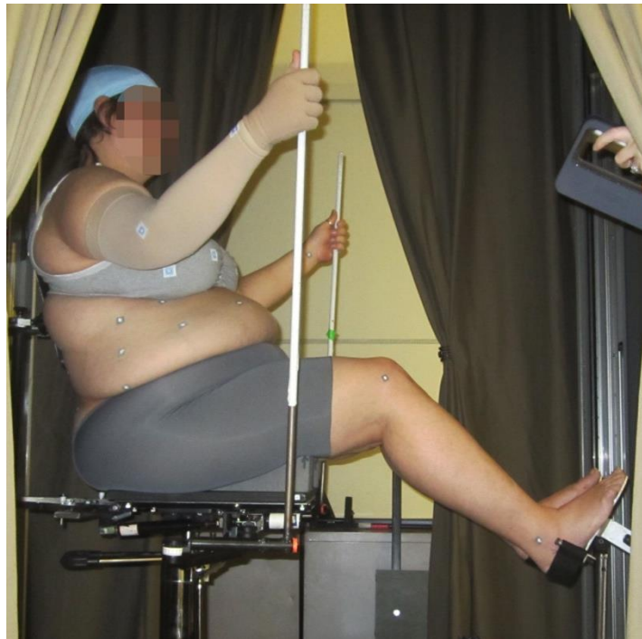
Figure C18. Participant in full-body scanner seat in automotive posture with investigator also using a hand-held scanner to record the shape of the lap area
