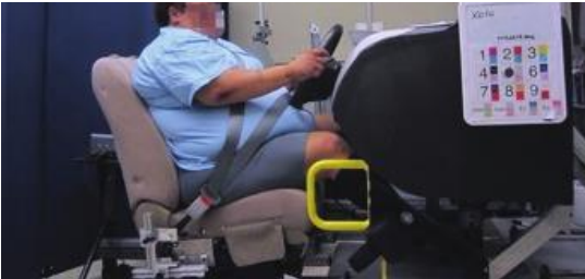
Figure 24. Photos showing lap belt fit for a range of occupant sizes (stratified by BMI classification).
