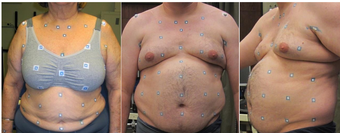
Figure C6. Torso grid markers stamped on participants' skin and taped to sports bra
