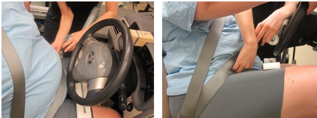
Figure 10. Palpating a participant's ASIS using the tool to locate the ASIS points in the driver mockup.
