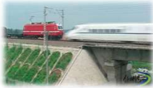
Figure 2.2.41 200 km/h Speed Passenger and 120 km/h Speed Truck Intersection Test (Photo from http://home.rails.com.cn/ )
