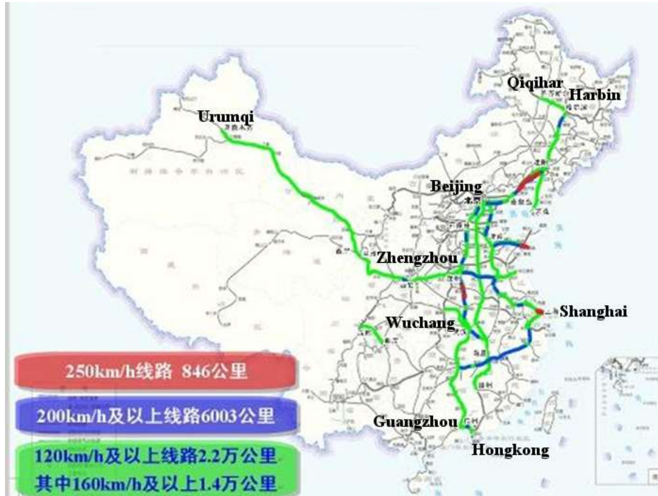
Figure 2.2.6 Summary of the Existing Railways after the Sixth Speed Upgrade (Green line: >120 km/h, total 22000 km; Blue line: >200 km/h, total 6003 km; Red line: >250 km/h, total 846 km) ( http://news.huoche.piao.com )
