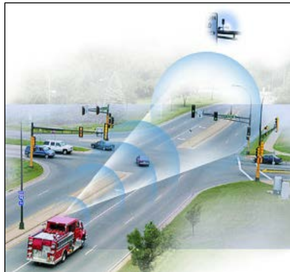
Figure 2. Illustration. Connected vehicle technology used to preempt traffic signals for emergency vehicles. (Source: U.S. Department of Transportation.)
