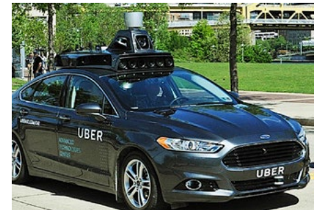
This automated vehicle is prepared for pilot testing. Note the array of sensors and communications devices.
