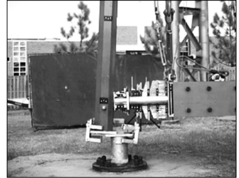
Just after the moment of impact, high speed video shows the simulated vehicle causing the breakaway device to separate.
