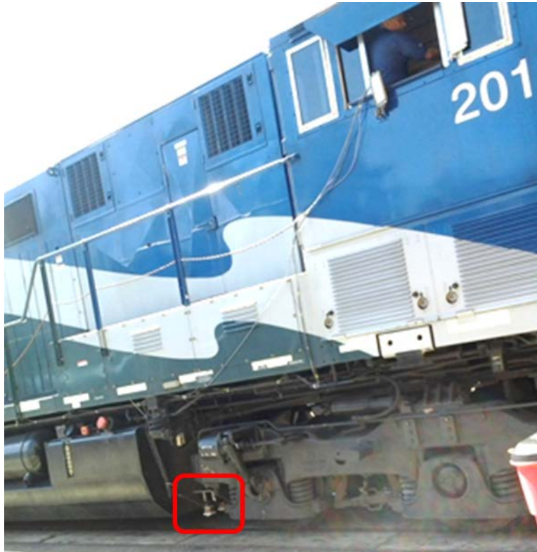
Figure 7. The transmitting coil mounted between fuel tank and wheels
