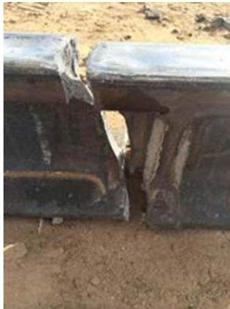
Figure 16. Details and images of the three broken rail occurrences during the TTC tests
