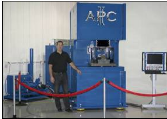
Figure 3. 100T LFW System Developed by APCI ( courtesy APCI )
