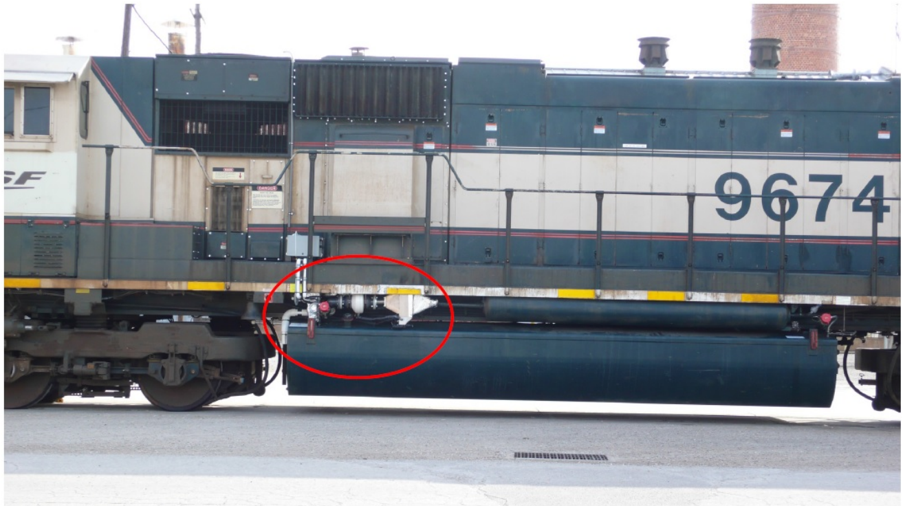
Figure 13. BNSF SD70 MAC locomotive # 9674 with installed DVRU in Topeka yard
