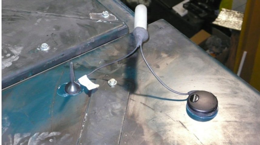
Figure 12. A GARMIN GPS and a GSM antenna installed on the roof of the locomotive
