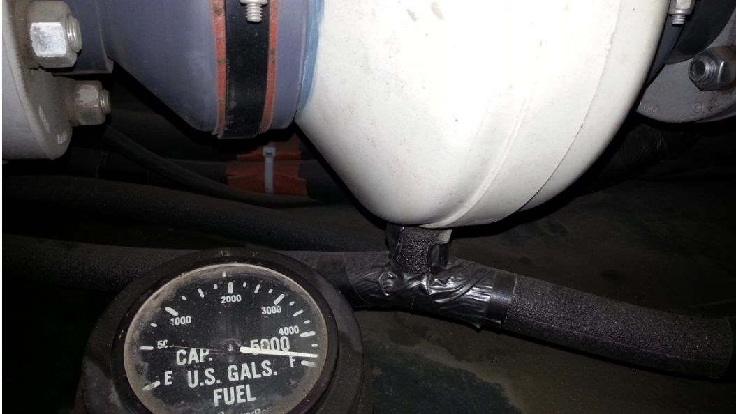
Figure 34. Locomotive # 9674 tank fuel gage showing a nearly full tank
