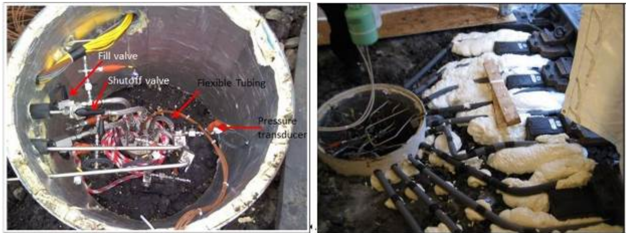
Figure 23. (left) Vault Interior Details (right) Tubing Support Insulation
