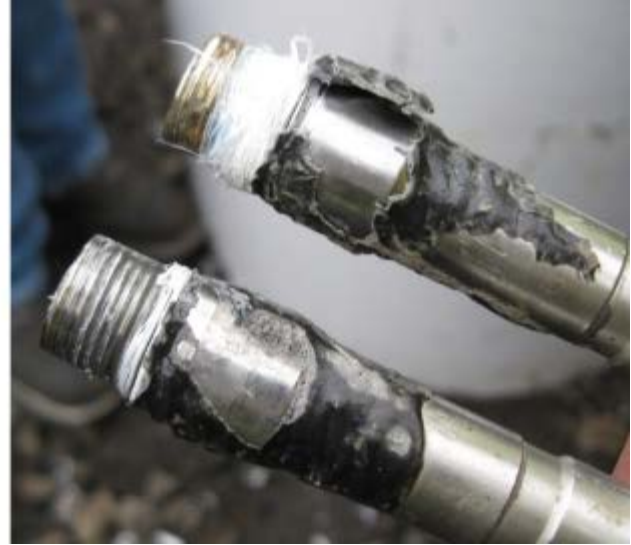
Figure 14. Damaged Tubing Ends
