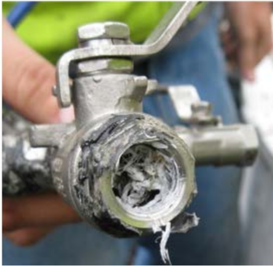
Figure 14. Damaged Tubing Ends
