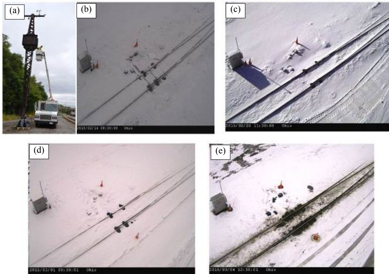
Figure 30. (a) Overhead Camera and Anemometer Setup on Old Catenary Tower (b) Feb. 14, Initial Overhead Photos show five Switch Plate Heating Systems Working (c) Feb. 20 after heavier snow (d) Mar. 1 system still working (e) Mar. 4, switch plates are clear
