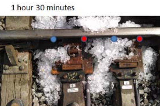
Figure 20. Ice Test at Conclusion of First Installation Phase
