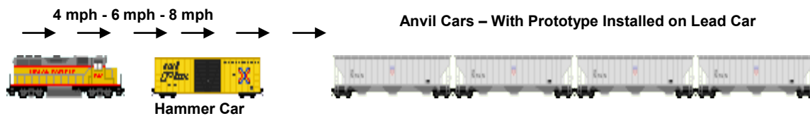
Figure 4. Impact Test Consist Setup
