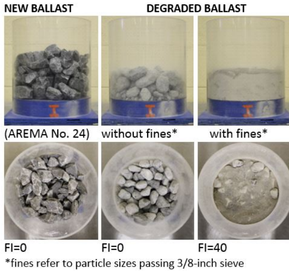
Figure 3. Side and top views of ballast aggregate packing
