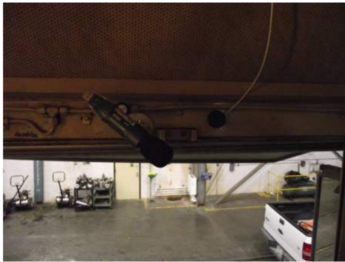
Figure 18. SPL Data Logger (conductor's side)
