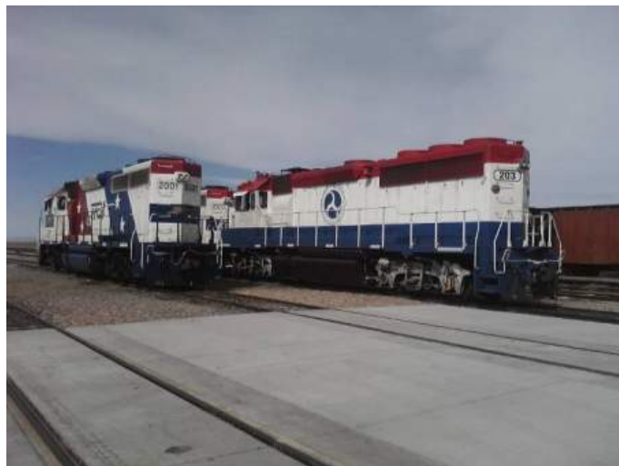
Figure 19. The 2001 Locomotive during Self-Load Testing at TTC
