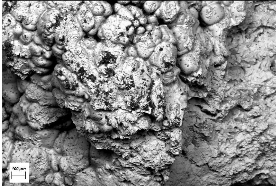
Figure 7. Gas Porosity in a Low Performing Charpy Impact Specimen
