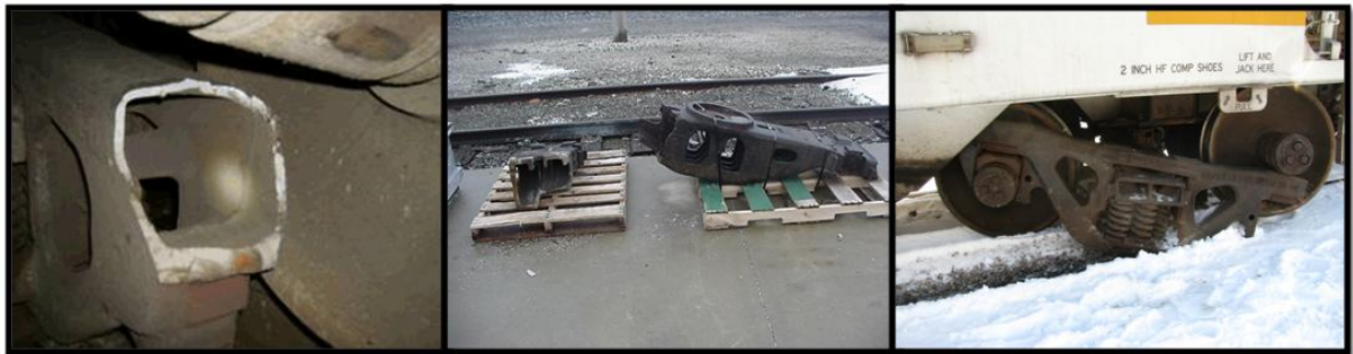
Figure 1. Examples of Brittle and Fatigue Failure in Truck Castings
