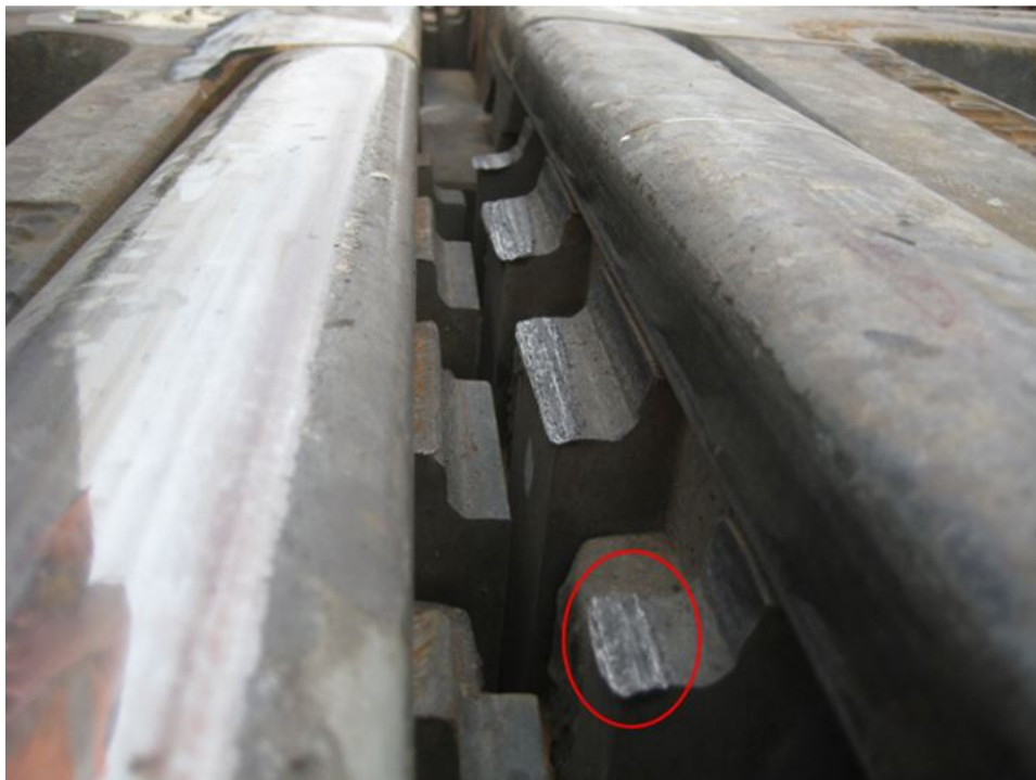
Figure 99. Wheel flange marks on the split spacer fastened to the rising guardrail
