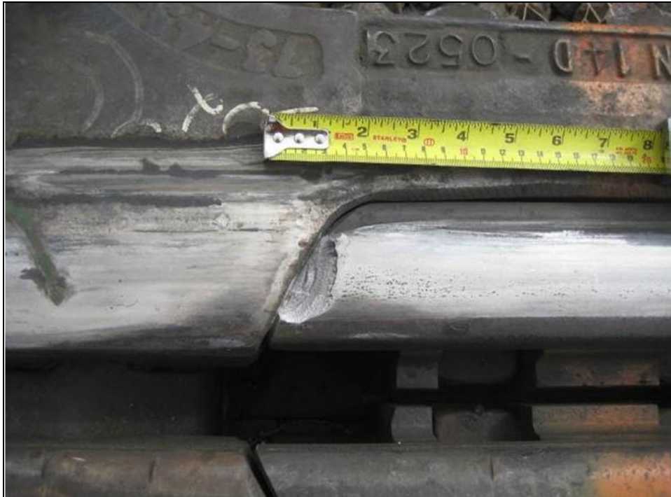
Figure 104. Chipped leg rail at the southwest frog was slotted
