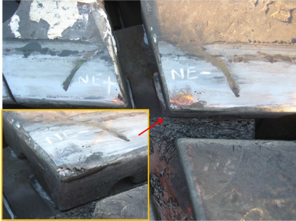
Figure 101. Casting corners were ground as required to remove metal flow
