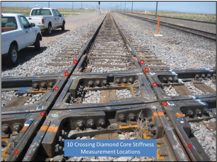
Figure 71. Locations of the 10 (5 on each rail) vertical track stiffness measurements taken at the core of the crossing diamond for each test case
