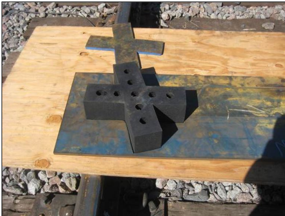
Figure 22. The solid rubber flangeway spacer tile embedded in the full-coverage rail seat Getzner Type B pad
