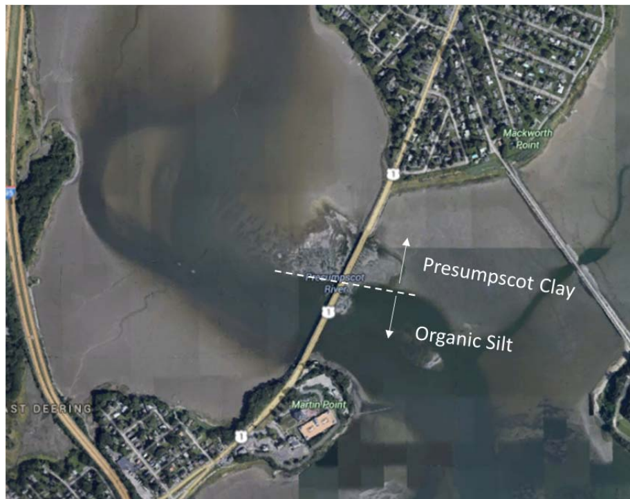
Figure 5.5: Aerial photograph of the Martin's Point Bridge site illustrating the effect of the Presumpscot River on the subsurface material (Google Earth, 2014).
