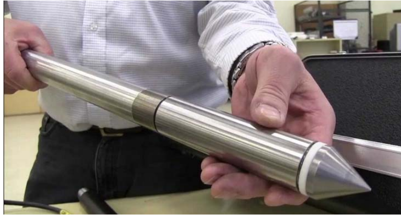
Figure 3.2: Image of a 1.4" diameter cone penetrometer showing the cone tip, pore pressure filter element, and friction sleeve (Vertek, 2014).
