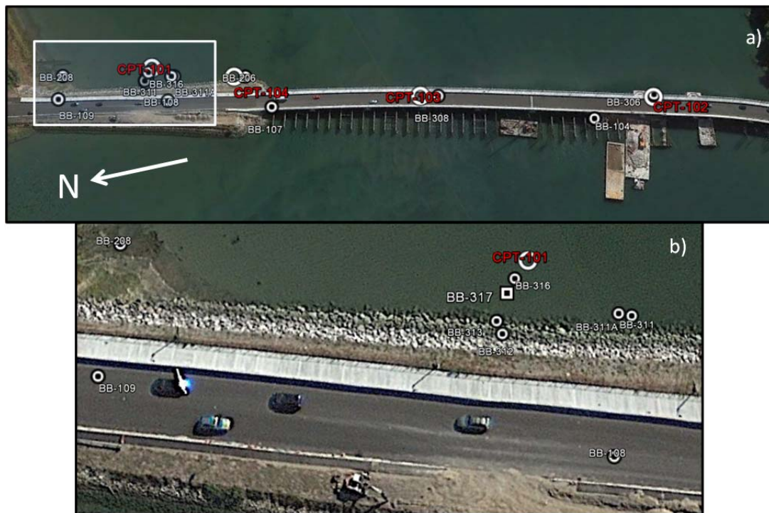
Figure 5.3: Aerial view of boring and CPTu locations along the a) entire length of the bridge b) Falmouth side bridge approach for the newly constructed Martin's Point Bridge (Google Earth, 2015).
