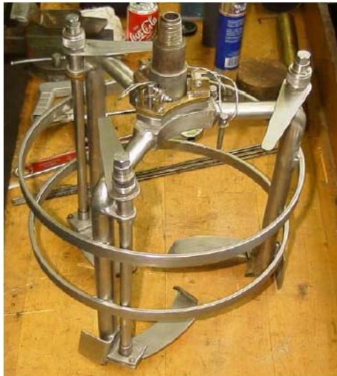
Figure 3.9: Sherbrooke block sampler (from Landon, 2007)
