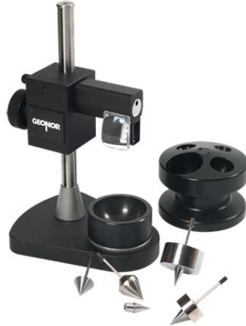
Figure 3.10: Geonor fall cone apparatus (from Geonor, 2010).
