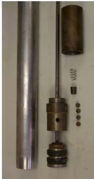
Figure 3.7: Modified Shelby tube fixed piston sampler with a 5^{\circ} machined cutting angle (from Landon, 2004).
