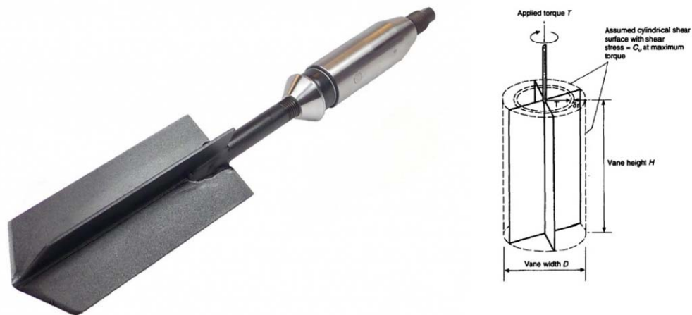
Figure 3.6: Image of field vane (left) and theoretical failure plane used for the calculation of undrained shear strength (right) ( www.gouda-geo.com and www.igeotest.com ).
