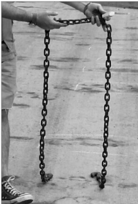
Figure 8.7 Chain drag test to detect delamination
