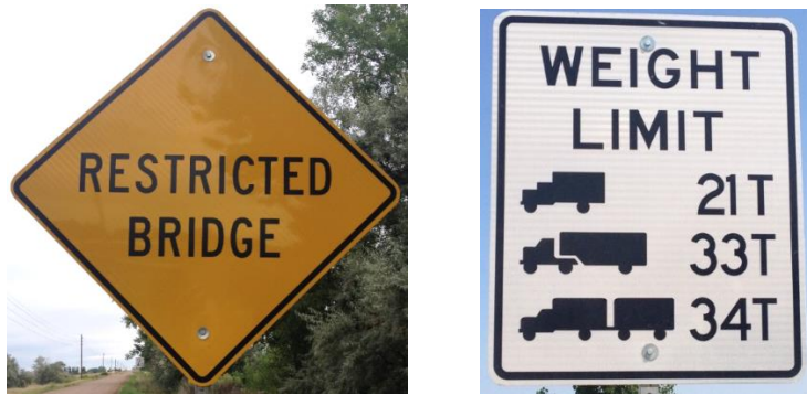
Figure 8.2 Advanced warning sign and load posting
