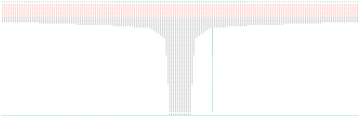
Figure 6.1 Output from the undamaged cross-section generator subroutine in Excel
