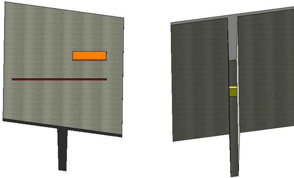
Figure 8.22 Left: view from top of Girder C with most severe cracking and delamination instances. Right: view from bottom of Girder C with most severe spalling instance
