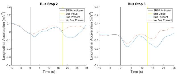
Figure 23. Comparison of driver longitudinal accelerations approaching the bus stops indicated via in-vehicle message. (Bus Stop 2 on left, Bus Stop 3 on right).
