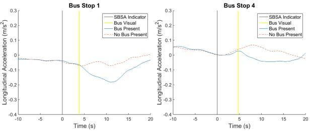
Figure 22. Comparison of vehicle longitudinal accelerations approaching the bus stops indicated via roadside sign. (Bus Stop 1 on left, Bus Stop 4 on right).
