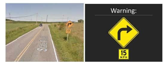
Figure 17. Location of (a) curve advisory warning and (b) in-vehicle display of curve advisory speed sign.
