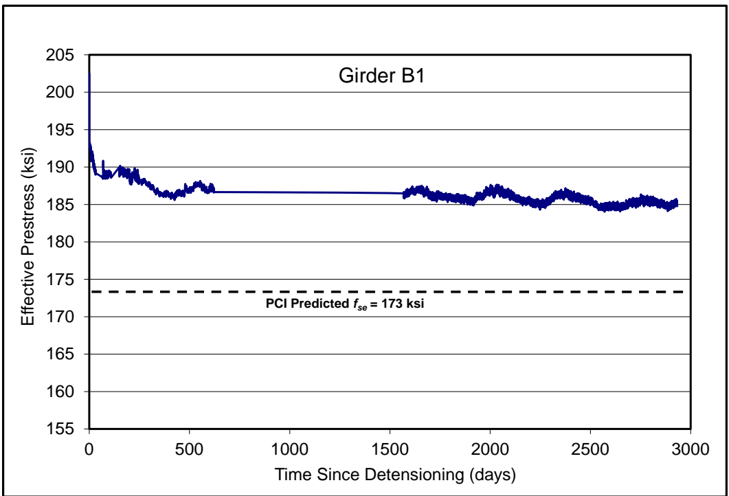
Figure 3.2: Effective Prestress Over Time for Girder B1
