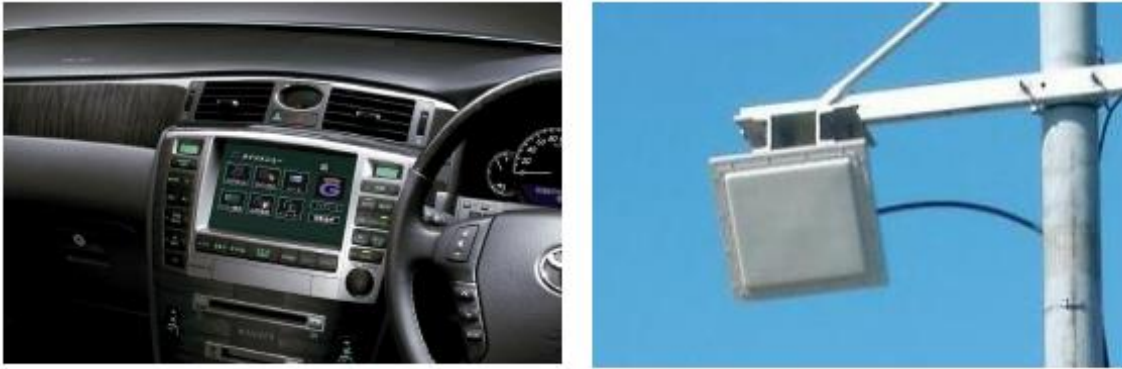
Figure 3-15. An ETC2.0-compatible car navigation system (left) and ETC2.0 roadside equipment (right) (Source: MLIT) [44]
