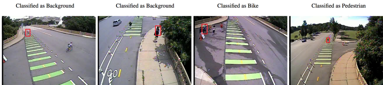
FIGURE 6. Examples of false detections of the cascaded detector. Column headings show the classification results of the detector. Low resolution of far objects, and/or partial occlusion are main reasons of the failure cases.
