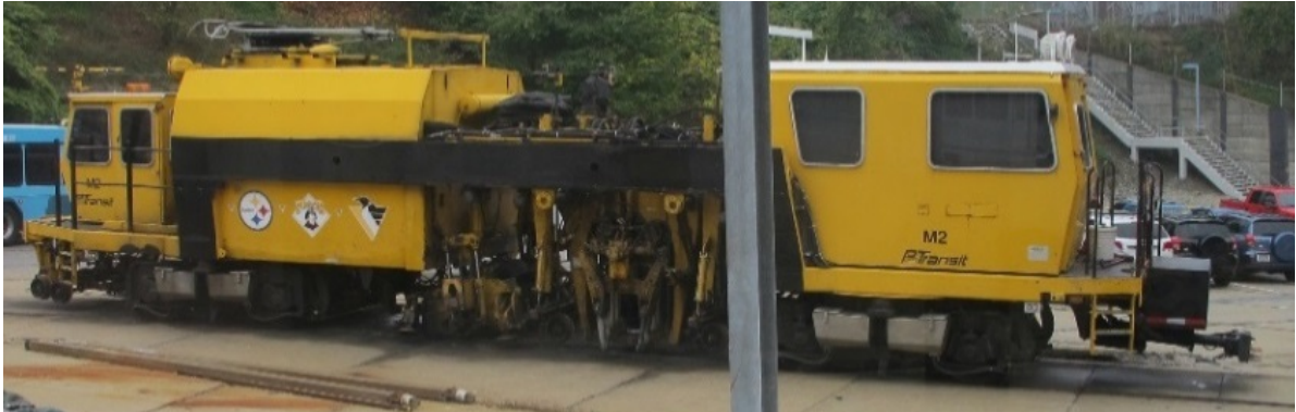
Fig. 15. The tamping machine used on the light-rail system.
