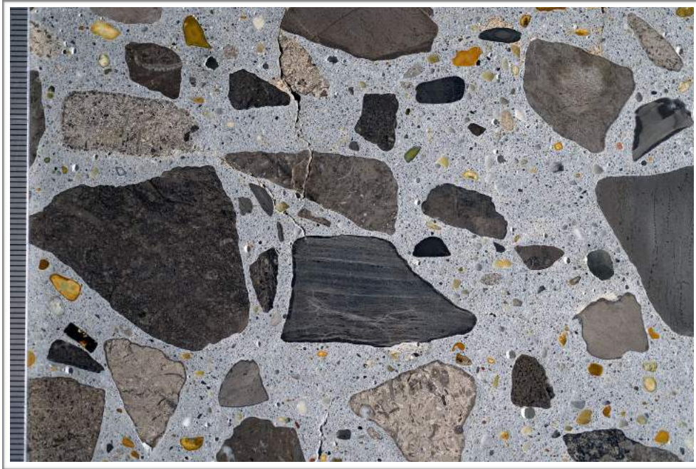
Figure B11. Photograph of the polished surface showing overview of coarse aggregate; scale in millimeters.
