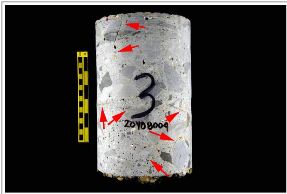
Figure C6. Photograph of the side of the core showing overview of cracks (red arrows). The yellow scale is ~ 150 mm (6 in.) long.
