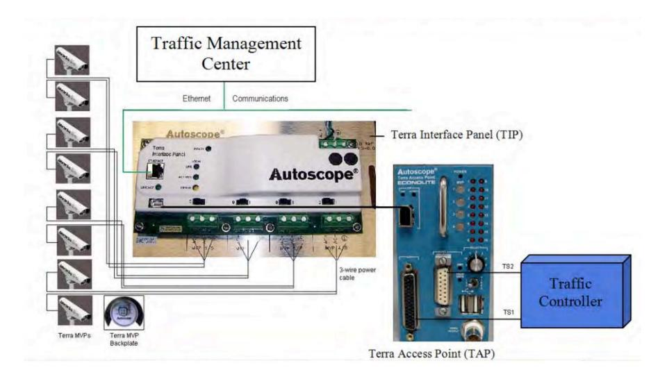
Figure 9 The Solo Terra Autoscope system components
