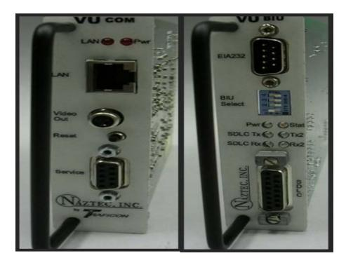
Figure 12 VU COM and the BIU for TS2
